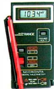
Basic, rugged and compact. Take it along or keep it handy in your toolbox, vehicle glovebox, desk or kitchen drawer. The continuity buzzer checks fuses, cords, more. Auto-ranging/manual. Recessed controls, low-battery and over-range indicators. Measures DC volts, AC volts and resistance.  $4\frac{1}{2} \times 2\frac{3}{16} \times 3\frac{3}{8}$ ". With case and batteries. 22-169 ..... 27.99
