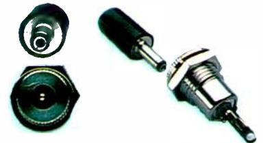
(Fig. B) Panel-mount DC power jack and plug
