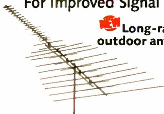
**LP-210 antenna.** One of our best VHF/UHF/FM antennas. Featuring advanced log periodic design that produces a visibly improved picture and adds much greater depth to FM-stereo broadcasts. Receives VHF/UHF/FM signals from distances of over 210 miles\*. Extra-long 180" boom with 57 receiving elements. 15-2166 ..... 129.99
