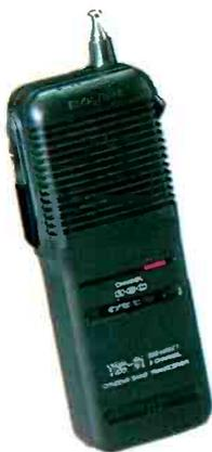
**Three channels, 300 mW, battery test button**
