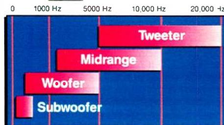
Speaker drivers and the typical frequency ranges they are designed to reproduce include the **subwoofer** (25-250 Hz), **woofer** (50-5,000 Hz), **midrange** (1,500-10,000 Hz) and **tweeter** (5,000-20,000 Hz).
