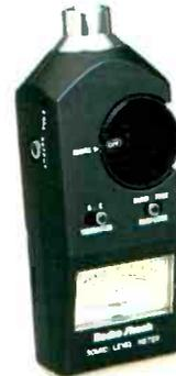
Reads to 126 dB SPL with slow or fast response for checking peak and average noise levels. Seven ranges. Electret mike. Requires 9V battery. **32-2050 . . . . . 31.99**
