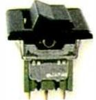
**Subminiature rocker—snap-in mount.** Solder lug terminals and silver contacts. Rated 6A at 125VAC. 0.453"-wide black rocker and black bezel. (on)=momentary.
