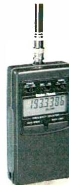
Accurate! Shows frequency of transmitter or RF source from 1 to 1300MHz. Confirms RF output from cordless phones, CBs, RC toy remotes, radio/TV circuits. Hams can use it to set a VFO precisely. Switchable backlight, selectable slow (1.28 sec.) or fast (128mS) update and 50-ohm or high-impedance input via BNC connector. Hold freezes display for easy reading. Add 4 "AA" alkaline or Ni-Cd batts. or AC adapter/charger #273-1455. (TSP) **22-306** . . . . . **99.99**
