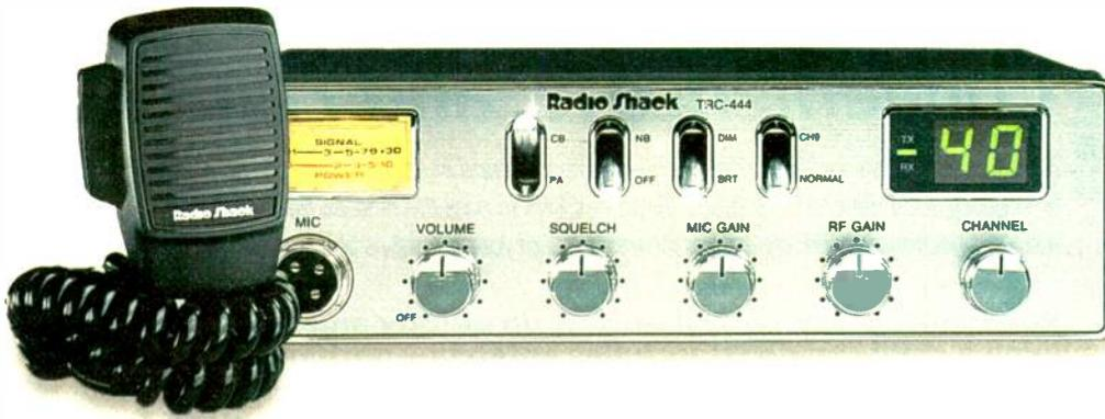
**Deluxe Classic Series mobile CB with microphone gain control, screw-on mic connector, and analog signal/power meter**
