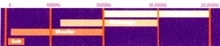
Speaker drivers and the typical frequency ranges they are designed to reproduce include the **subwoofer** (25-250Hz), **woofer** (50-5,000Hz), **midrange** (1,500-10,000Hz) and **tweeter** (5,000-20,000Hz).
