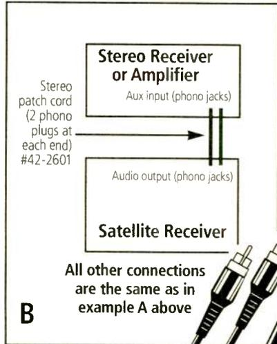
Example B uses a patch cord with phono plugs (also called RCA plugs) and a coax cable with F-type connectors
