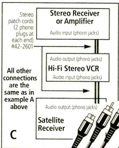
Example C uses two patch cords with phono plugs and a coax cable with F-type connectors. (Optional S-video cable shown at left)
