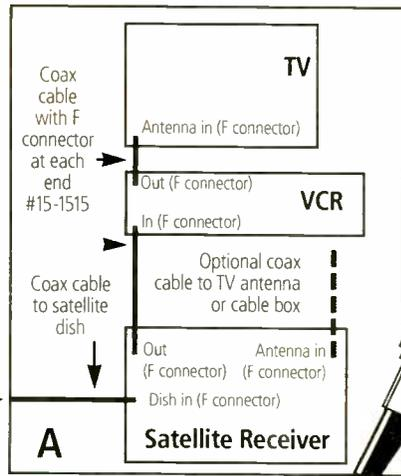
Example A uses a coax cable with F-type connectors
