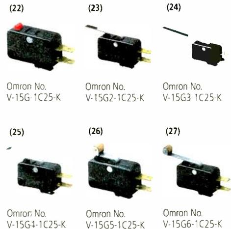
SPDT, 0.187" quick-connect terminals. Rated 15A/125VAC.
