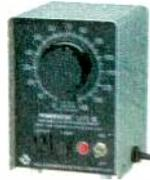
**L21C.** Ideally suited for use in applications requiring a portable variable AC voltage source. Designed to operate from a 120VAC 50/60Hz source and deliver an output of 0-140VAC at 4.5A. Maximum KVA rating is 0.63KVA. A grounded NEMA cord-plug assembly, on-off switch, pilot light, output receptacle and fuse provide maximum protection and safety. Mfr. warranty: one-year limited. 7 1/4 x 5 1/2 x 5 1/2". **900-8682**..... **249.99**
