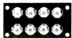
**Board with 8 standard-type phono jacks.** Readily accepts solder for solid electrical connections. 274-370 ..... 2.29
