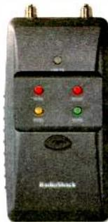
**Test coax and phone cables for shorts, opens and reverse polarity**
