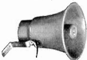
MODEL HU-12 Power . . . 3 watts Impedance . . 8 ohms Frequency . . 375 to 9000 Length . . . 7 1/2 in. Diameter . . 6 1/4 in. Air Column . . 13 1/2 in. List Price . . $23.00
