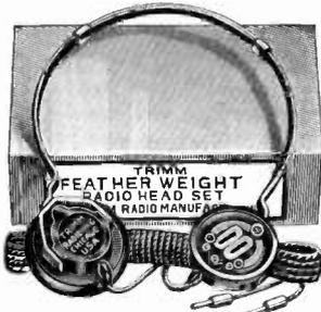
The world famous TRIMM Featherweight. Recognized as a leading quality headset. Weighs 4½ oz. complete with two units, 5-foot moisture-proof wear-resisting cord. Bakelite shell and cap. Magnet of highest quality cobalt steel alloy. Pole pieces of finest magnetic iron. Coils especially impregnated. A custom-built phone throughout. Standard resistances.
