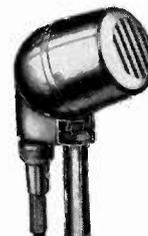
Attractive, dependable, general-utility mike. Frequency response 50-7500 c.p.s., substantially flat. Output level 57 db below 1 volt/dyne/cm<sup>2</sup>. Exclusive E-V Acoustalloy diaphragm. Pressure cast case, with 22° fixed tilt.  $\frac{5}{8}$ "-27 thread. Built-in cable connector. Satin Chromium finish. Net wt., 12 ounces. Available in
