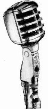
Moving-coil Dynamic Models are available in Hi-Z (direct-to-grid, 25,000 ohms) 50, 150, 250, or 500 ohms impedance. Low impedances balanced to ground. Crystal Models are Hi-Z.
