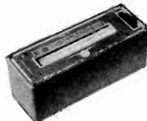
Model 105 Roll chart unit to be used in conjunction with Tube Tester Models 322, 322P, 322A, 322AP, 802N and 802NA. The unit is in a grey hammer-tone finish metal case with plastic window, designed to fit the test lead compartment.
