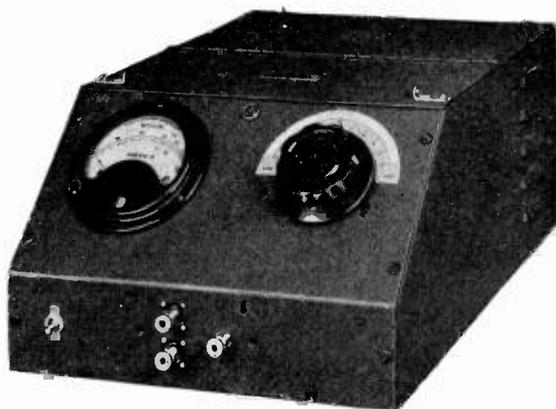
Capacitance Range: Capacitance values ranging between approximately 2-1000 mmf. may be checked against a standard to an accuracy of a few tenths of one mmf. if the Q of the capacitor is high.
