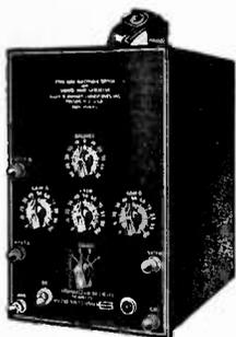
★ The Du Mont Type 185-A Electronic Switch may be used in conjunction with any oscillograph to observe two related or unrelated signals simultaneously on the screen of the cathode-ray tube. The zero axes of the two signals may be displaced for individual study of either pattern. The two patterns may also be superimposed for comparative studies. A typical application is the use of one channel for the signal to be studied while using the second channel for a timing signal.
