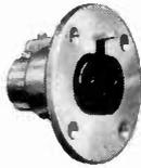
Flange is 2" in diameter, drilled with four holes to take #4-40 oval-head mounting screws, 90° apart on a radius of  $\frac{1}{8}$ ". Made of die-cast zinc, cadmium plated. Latch Locking Device is operated from panel front.
