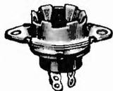
Economical chassis receptacles for connecting shielded or unshielded cables having from 2 to 6 conductors (for 2 wire cable use 3 contact unit and leave 1 contact unwired). Black Bakelite element; steel mounting plate. Can be mounted on surface or behind chassis or panel in 7/8" D. hole; 5/32" screw holes on 1-1/4" centers. Use with long shell cable connector above for a fully shielded connection.
