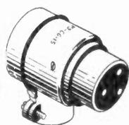
Has Split Shell and all other "Type P" features found in "Type P-15. 90° Plug" except cable connection, which is an Integral Clamp for  $\frac{1}{2}$ " or smaller cable. Made of cast aluminum alloy, finished in tin plate. New, heavier clamp.
