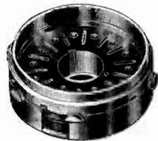
Designed for television viewing tubes, oscilloscopes and other cathode-ray tubes. Provides means of grouping leads within the socket housing and bringing them out radially in a neat, unit-cable form, reducing the space required to a minimum. Grouping of the wires in the enclosed raceway eliminates flexing at solder terminals, minimizing breakage.
