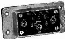
Mounting flange is  $3\frac{3}{8}$ " x  $1\frac{1}{4}$ " and shell extends  $\frac{3}{8}$ " from the mounting surface forward. Coaxial contacts extend  $\frac{3}{8}$ " to the rear from the mounting surface. Shells provide for mounting with four No. 6 oval head machine screws. Material is aluminum.
