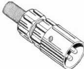
Type XL-12 plug has alignment rib in addition to polarizing groove. Cable accommodation is  $\frac{3}{8}$ . Insert is removable for soldering or inspection. Overall dimensions:
