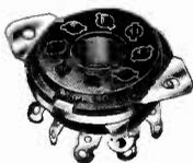
Sharp nibs on mounting plate score chassis during riveting, breaking thru any oxidation for a perfect ground. Designed for bottom mounting in 1-1/8" round hole. Two 5/32" diameter mounting holes on 1-1/2" centers.
