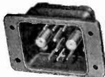
The DPB Plugs are similar to the Type DPD, differing in the same respect as the DPB Receptacle differs from the DPD. They are mounted with four No. 6 Oval Head Machine Screws. Standard finish on all DPB shells is tinplate and clear lacquer. Other finishes by special order.
