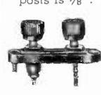
Cat. No. 21-S. All-molded Bakelite, non-removable tops. One post is completely insulated. One mounting screw 6/32" x ¼" long. Ground post is second mounting screw. Base is 2" long, 11/16" wide and 3/16" thick. List Price \$0.70 ea.
