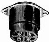
For rectifier and other tubes with base diameter of 1.156". Socket is set at the bottom of a deep molded Bakelite shell. Heavy steel mounting plate molded into shell has 5/32" diam. mounting holes on 1-7/8" centers. Socket mounts from above or below in 1-1/2" round hole.
