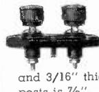
Cat. No. 21-R. All-molded Bakelite, non-removable tops. Both posts completely insulated. Center mounting screw 6/32" x ¼" long. Base is 2" long, 11/16" wide and 3/16" thick. Center distance between posts is 7/8".
