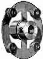
The sides of coupling are insulated from each other, allowing instruments in gang to be operated as independent electrical units. Bakelized canvas with brass bushings for  $\frac{1}{4}$ " shaft. Four rust proofed and hardened steel set screws provide against shaft slipping. Overall diameter  $1\frac{1}{2}$ ".
