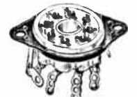
Body molded from transparent Amphenol "912-A" (polystyrene). Remarkable LOW-LOSS properties provide greater efficiency for ultrahigh frequency work than has ever before been possible. (Caution—solder fast! Do not heat beyond 200° F. Requires 1 1/4" hole; 1 1/4" mounting centers.)
