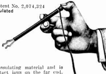
The long tube is of insulating material and is fitted with spring contact jaws on the far end. The jaws are operated by a push of the thumb on the near end. Wire is quickly and easily connected in a hole in the insulator knob binding post on the near end.
