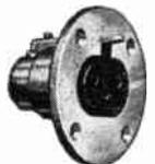
Flange is 2" in diameter, drilled with four holes to take #4-40 oval-head mounting screws, 90° apart on a radius of  $\frac{11}{16}$ ". Made of die-cast zinc, cadmium plated and finished in clear lacquer. Latch Locking Device is operated from panel front.
