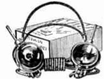
The choice of countless users... the original TRIMM headset. Double unit watch case type. Bakelite cap and shell, forged magnet of chrome steel, impregnated coils, 5 foot moisture-proof wear resisting cord, entirely concealed terminals. Fabric-covered wire headband. Standard resistances.
