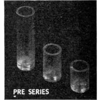
For ultra high frequency work, where very low losses are essential, these small Victron coil forms will be found extremely useful. They can be readily drilled and grooved with ordinary tools, and firmly cemented with National Coil Dope without impairing electrical characteristics.
