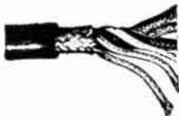
Conductors all color-coded. Braided with tinned copper shield. Heavy Jacket Tough Black Polished Rubber applied overall. Will withstand severe service. Adaptable to carbon, condenser, and moving coil microphones. **POSITIVELY WATERPROOF**—excellent for field microphones.
