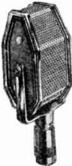
Answering the demand for a high quality velocity microphone at a competitive price, Amperite presents models RAH-RAL. Excellent for both speech and music. Eliminates feedback. Has a frequency range of 60 to 7500 cps. Output, —68 db. Unaffected by temperature or humidity. Unusually rugged. Triple shielded, and fitted with heavy shock absorber. Shipping weight 5 lbs.
