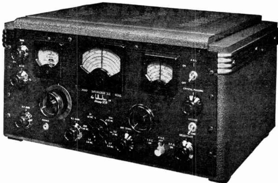
**THE "SKYRIDER 32"** has two stages of preselection—high fidelity audio—calibrated band spread—micrometer dial on main dial control—heavy gauge steel cadmium plated chassis—standard size relay rack panel  $\frac{1}{8}$ " thick—machine tool gray wrinkle finish cabinet well ventilated and attractively designed.
