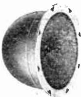
As used in 15" coaxials. Designed to reproduce the high frequencies from 4,000 to 15,000 cps., when used with dividing network (such as A40-1) and suitable low frequency speaker. Impedance, 16 ohms. Overall diameter, 5 1/2". Depth, 3 5/8". P.M. design.
