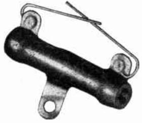
"Wirewatt" and "Brown Devil" center-tapped resistors especially designed for use across radio transmitter tube filaments to provide an electrical center for the grid and plate returns. Should be connected as closely as possible to the tube socket. Center tap accurate to plus or minus 1%.
