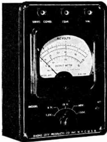
This instrument has non-inductive constant input impedance of 4,000 ohms for all five ranges. All resistors are precision wire wound, non-inductive and accurate within 1%.
