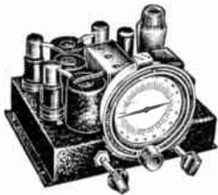
A low-cost, T.R.F. receiver that is surprisingly simple and easy to build and yet provides remarkable performance. Operates from 110-volt, 50- to 60-cycle lines and covers Broadcast band between 530 and 1600 kc (187 to 365 meters).
