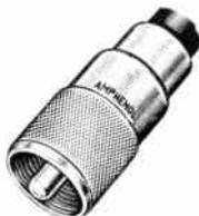
These connector plugs are specially designed to accommodate coaxial and twinax cables. Low-loss, mica-filled bakelite and polystyrene insulations. All surfaces are heavily silver plated. The small size of these Amphenol connectors makes electrical discontinuity extremely slight—and with the dielectrics butted to each other and to the Copolene core of the cable, there is minimum air space so that constant characteristics are maintained.
