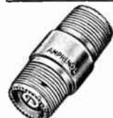
Straight junction connectors, completely assembled with socket contacts on both ends. It is used for joining two cables (with two No. 83-1SP, 83-22SP, or 83-2SP connector plugs) or for repairing damaged cable. Dielectric is pure polystyrene. There are no air spaces.
