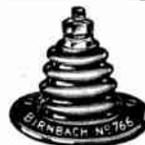
Base measures 2" dia. with 3 holes on a 1 1/2" circle, for No. 6 screws. Supplied complete with 12-21 nickel-plated brass screw and nuts. The No. 766J has a No. 403 Jack. Available white or brown glaze.
