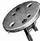
The "XS-2" is a special crystal socket designed to conserve space and provide a low loss mounting for standard crystal holders. Made with heavy-duty spring contacts and mounted on glazed Isolantite. Can also be mounted inside "SWF" coil forms for changing coil and crystal in one operation. Overall diameter  $1\frac{1}{16}$ ".
