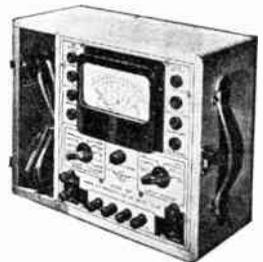
CHECK THESE FEATURES: Dual D.C. sensitivity of 20,000 ohms per volt and 1,000 ohms per volt. A.C. sensitivity of 1,000 ohms per volt. Wide scale 4 1/2" meter with movement of 50 microamperes. Readings as low as 1 microampere. All multipliers matched and 1% accurate. Three ohmmeter ranges. Center of ohmmeter scale 40 ohms. Readings as low as 0.25 ohms. Batteries are readily accessible . . . can be replaced merely by releasing spring clamp. No soldered terminal connection to batteries.
