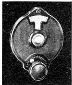
"Velvet Vernier" Dial, Type B, has a compact variable ratio 6 to 1 minimum, 20 to 1 maximum drive that is smooth and trouble free. An illuminator is available. The case is black bakelite. 1 or 5 scale. 4" diam. Fits  $\frac{1}{4}$ " shaft.
