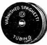
A flexible tubing, heavily varnished, in attractive colors. Average dielectric strength, 5000 volts. Will accommodate from No. 10 to No. 18 wires. Furnished in one length—20 feet long on handy spools.
