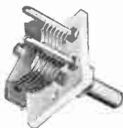
For tuning or trimming on high frequencies. Cadmium plated soldered brass plates. Isolantite. Base mounting, single hole panel mount, or panel mounting with bushings. 140 mmf. size 1 3/8" high x 1 1/8" behind panel.
