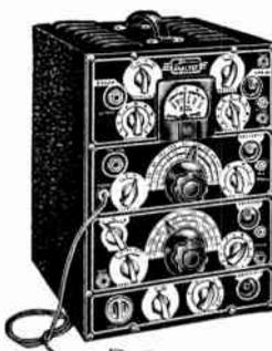
Five separate and distinct "channels" provide as many different functions; all controls are accurately calibrated with functions clearly indicated.
