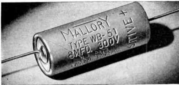
• Type WB capacitors are supplied in hermetically sealed aluminum tubes with waxed cardboard outer sleeves. They are suitable for all general applications within the specifications shown below. Particularly noteworthy are their excellent low-temperature characteristics. They may be obtained with radial strap for mounting, if desired, by specifying type WBR.
