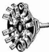
A compact inexpensive switch for many circuit applications. May be used as single pole single throw, single pole double throw, double pole single throw, double pole double throw, three pole single throw, three pole double throw, four pole single throw, four pole double throw. Non-shorting teeth. Flat construction requires only  $\frac{5}{8}$ " overall back of mounting surface. Supplied with aluminum shaft  $2\frac{1}{4}$ " overall. Standard bar knob included.
