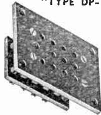
Socket Panel Assembly is 2 3/8" x 2" x 3/8" with a solder pot extension of 3/8". 4 mounting holes .120 drill size for No. 4 FH screws.
