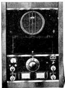
**SPC**, combination of 697 power unit, coil container (5 coil capacity) and 8" PM dynamic speaker. Rack panel, 3/16" x 15 3/4" x 19". Chrome strips included.
