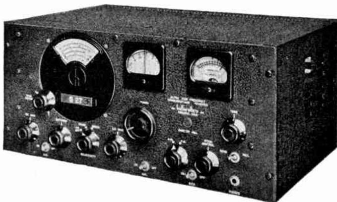
**T**HIS Frequency Modulation communications receiver covers 3 bands: 27 to 46mc; 45 to 84mc; 81 to 145mc. Switch changing from FM to AM reception. Acorn tubes in R.F. and converter system. High gain 1852 tubes in Iron Core I.F. stages. Beam power tubes in A.F. amplifier. Controls are: R.F. gain control. Band switch. Antenna trimmer. I.F. selectivity control and power switch.
