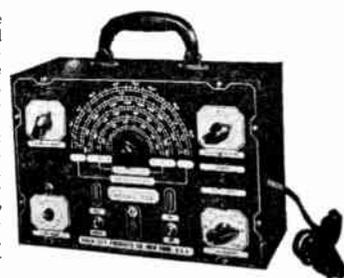
Self-contained modulation source is 400 cycles sine wave which modulates carrier at 30%. This frequency is available for external use. Provision also made for applying external modulation to signal. All coils not in use automatically shorted. Individual shielding of R.F. circuits, coil assembly and attenuator, in addition to overall steel case, chassis and panel. Attenuation in approximate microvolts by five step ladder attenuator, calibrated to 500,000.
