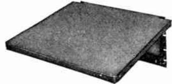
These standard tables are rigidly made of 1/4" thick furniture steel. The rounded front corners are of seamless construction and the flanges of the shelf are folded in to provide smooth edges underneath. They are securely mounted to regular 1/8" steel panels, size 10½"x19". They may be obtained in two sizes and finishes as listed below. The tables are 22" wide to give full working space across the front of the racks when mounted in place. Shipping weight is 35 lbs.
