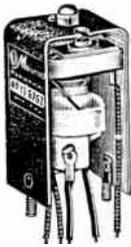
Special, close-coupled transformers for use in "Lamb" type noise-silencer circuits. Complete range of I-F frequencies available, with air or mica dielectric trimmers; air-tuned units are 2" sq. x 4 1/2"; mica-tuned units 1 3/4" sq. x 3 1/2".
