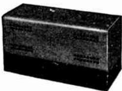
Rounded corners effectively streamline the covers on these units. Grille type ventilation gives them a modern appearance. Chassis stamped from one piece of cold rolled steel, with corners securely spot welded. Covers finished in slate grey, chassis in black ripple enamel. Chassis are drilled for bottom plates. Handles can be mounted at both ends of the cover at an addition of 42c net.
