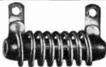
Designed to prevent unwanted ultra-high-frequency parasitic oscillations which occur in the plate and grid leads of push-pull and parallel tube circuits. The parasitics are suppressed, without loss of driving power.
