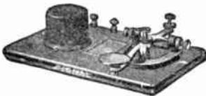
Designed for those who want a well made instrument to learn the code. Set consists of a key and high frequency buzzer mounted on a mahogany finished wood base equipped with binding posts. The code is printed on a plate and fastened to the base between the key and buzzer. Buzzer is adjustable.
