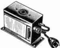
Designed for use in the most serious cases of radio interference from power lines and appliances. Provided with inductance as well as capacitance for thorough filtering action. Plugs into electric outlet. Radio set or interfering device plugs into receptacle of the filter. Especially desirable between device and line. Measures 4 x 2 3/4 x 3 1/2 in. 110-220v. A.C.
