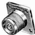
These are complete units. One-piece construction makes for easy soldering to connectors within box or chassis. Die cast zinc shell silver plated for conducting high frequency current. Low-loss, mica-filled bakelite dielectric. High conductivity copper alloy socket contact.
