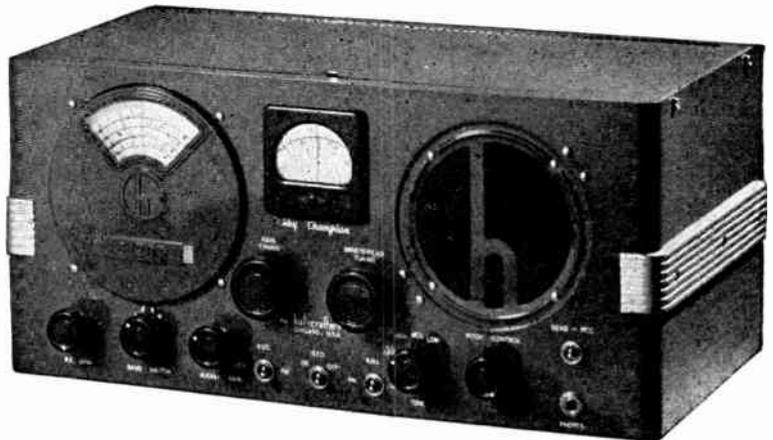
**FEATURES:** 9 tubes. Complete coverage (545 kc. to 44 mc.). Inertia tuning. Separate electrical bandspread. Beat frequency oscillator. Battery-vibrapack DC operation socket. Cabinet size—18½" long, 8½" high, 9¾" deep.
