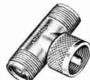
One-piece completely assembled units used for providing leads to additional equipment by means of an additional pin contact at right angle to the socket contact. Cast zinc silver plated. Polystyrene insulation assembled with liquid polystyrene to eliminate air spaces.
