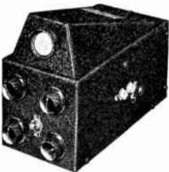
The Type CRM oscilloscope is mounted in a small steel cabinet (4 1/8" x 6 1/8" x 8") and uses a one-inch screen RCA-913 with 6X5 rectifier. Power supply and input controls are built in. A panel switch permits use of the built-in 60 cycle sweep or external audio sweep for securing the familiar trapezoid pattern for modulation measurements. **CRM**, less tubes,
