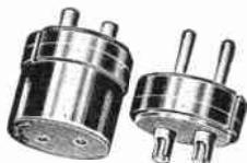
Inserts with thermocouple metal contacts have been designed to provide more accurate readings on thermocouple type instruments. The contacts are made of iron and constantan instead of bronze. These inserts can be used in any shell of corresponding size.
