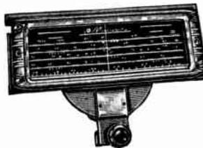
**9-INCH** Used on larger Meissner receivers; single-speed vernier mechanism; fits 3/4" shaft; for right or left-hand closing condenser. 4-band scale calibrated 537-1754 kc, 1.68-5.96 mc, 5.85-18.2 mc and 17.6-42 mc. 5-band scale has 133-408 kc band additional.
