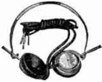
A superior headset in the lightweight low price field. Cap and shell of molded bakelite, chrome steel magnets, and weighs six ounces complete with two units, 4 1/2 foot cord and metal headband.
