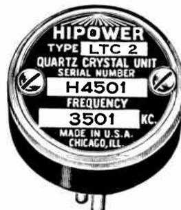
Consisting of an extremely active crystal with a temperature coefficient of 10 cycles or less per MC. per ° C. Mounted between NICKEL SILVER electrodes, in a molded Bakelite holder, for plug-in mounting in a five prong tube socket.
