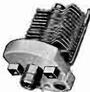
For S.W. and ultra-S.W. For I.F. tuning, trimming R.F. coils or gang condensers, general padding, etc. Constant capacity under any conditions of temperature or vibration. Size 100 mmf.  $1\text{--}7/32$ " x  $15/16$ " x  $1\text{--}7/32$ ". Isolantite base. Cadmium plated soldered brass plates.
