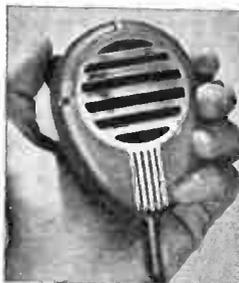
Fits comfortably in palm of hand. Light, compact. Takes minimum space in portable equipment. Die cast case in Iridescent Gray with satin finish grille. Excellent response. Output level; 32.5 db below 1 volt for 10 bar speech signal. Specially designed "ON-OFF" switch. Complete with removable suspension hook, 7 ft. shielded cable and spring cable protector. 3 3/4" high, 2 3/4" wide, 1 1/4" thick. Shpg. wt. 1 lb.
