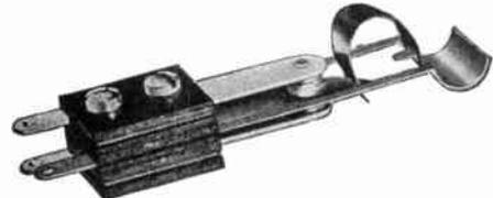
This type of open blade switch is designed for cam actuation. Switches weigh approximately 1 oz. Size is 3" x 11/16" x 1/2". Two 6-32 screws provide for mounting.
