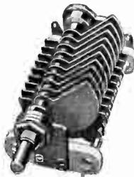
Exceptional unit for ultra-s.w. receivers and transmitters particularly compact transmitters. Plate spacing—.0715". Great for tuning crystal controlled transmitter amplifier stages or for neutralizers up to 1000 volts. In midline (MX) and straight line cap. types (SX).
