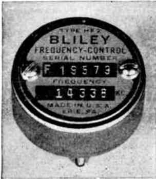
Frequency multiplication in 2½, 5, 10, or 20-meter transmitters is minimized with the HF2 unit for 20 meters. This fully dependable mounted crystal has high activity comparable to lower frequency crystals and is, therefore, easily excited. Physical ruggedness is accomplished by employing the harmonic vibrating principle. The crystal can be used in any conventional triode, pentode
