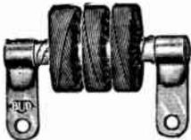
This newly designed choke is for use with the new medium power transmitting tubes in high and ultra-high frequency circuits. Three lateral wound pies on 1/2" diameter Isolantite core. Heavy strap leads. Size 3/4" diameter by 1 1/2" long. Inductance, 2.5 M.H.; D.C. Res. 16 ohms; Current Cap. 250 MA. continuous; Dist. Cap. 2 mmfd.
