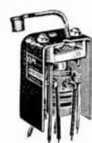
Combined oscillator coil and input I-F transformer in one shield; for replacement use and new set construction. Designed to cover broadcast band from 190 to 550 meters with a 365-mmf tuning condenser. Double-tuned with ceramic-base trimmers; shield is 2" x 2" x 3".
