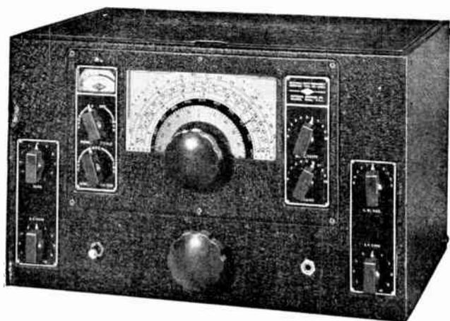
**NC-100A** — complete with tubes. AC model — 10" speaker in cabinet.
