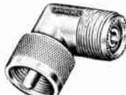
One-piece completely assembled units. High conductivity copper alloy pin contacts on one end, socket contacts on opposite end, assembled without solder. Pure polystyrene dielectric. No air spaces inside the unit. Plugged, die-cast zinc construction, heavily silver plated.
