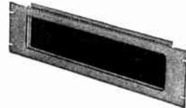
These panels are made so that the meters may be recessed from the front of the panel. Meters are protected by a plate glass insert, allowing ¼" clearance in back of panel. A blank bakelite sub-panel is provided. The clear sub-panel space is 4½"x15" on the 19" wide panel which is sufficient for 4-3" meters. On the 24" and 30" wide panel the clear sub-panel space is 5¼"x20" and 5¼"x26" respectively.
