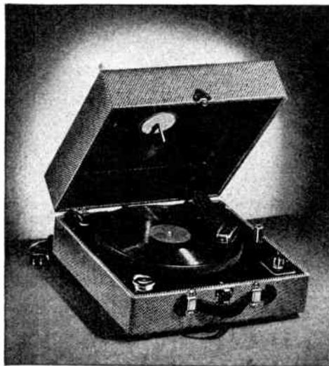
Model No. 101 phonograph unit is a record playing device for either ten or twelve inch phonograph records and it comprises a 78 R.P.M., rim drive phonograph motor with a ten inch flock covered turntable. The phonograph pickup is of the off-set arm type with a crystal cartridge. Output for 500,000 ohm load.
