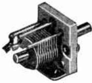
For efficient tuning of ultra-high frequency circuits. Alsimag 196 insulation. Soldered brass plate assemblies, cadmium plated. Rear shaft extension for ganging. Three way mounting. Mounting space 1 1/2" x 1 1/4".
