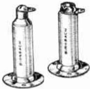
These (steatite) pillar insulators have great tensile strength with extremely low losses at very high frequencies and are glazed on the outside to decrease surface leakage. They are tapped on both ends and are supplied complete with nickel-plated mounting base and top hardware.
