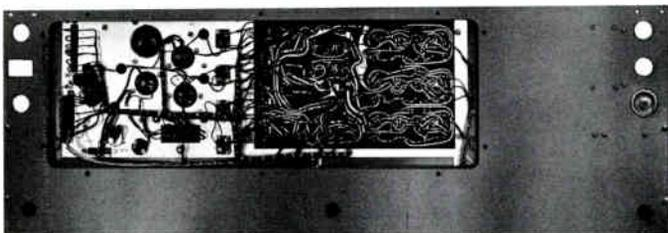
All wiring on the printed circuit board is accessible through a removable cover plate on the bottom of the console. The entire console is hinged to permit easy access.
