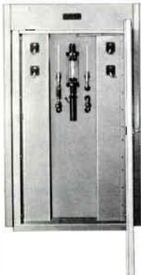
The Gates 50 kW water cooled dummy antenna is available either for medium wave or short wave application. The medium wave unit is essentially non-reactive in the 200-2000 kHz band, and does not usually require a matching network. Both models will easily handle a full 50 kW 100% modulated when provided with suitable water flow. Water of reasonable purity can be used; normal required flow is approximately 15 gallons per minute. Dual thermometers and flow meter
