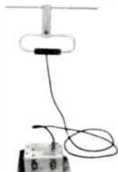
For remote indication of RF current. Consists of a carefully constructed pickup loop attached through a short coaxial cable to a solid state rectifier assembly. RF current is measured without breaking the main lead. No AC power is required. May be used with any good 1 MA DC meter. Power range: 250 watts to 50,000 watts. Frequency range: 540 kHz to 1600 kHz.
