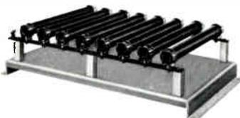
This unit may be used for any medium wave transmitter at a maximum power rating of 1 kW, 100% modulated. Consists of non-inductive resistors heavily banded together to arrive at correct load resistance. For 200 kHz to 2000 kHz. 20¼" x 12¾" x 5" high. Available in 50 ohm and 70 ohm models.
