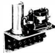
Replaces circuit breakers in current or older models, as circuit breakers are usually undependable for remote control. Tripping current adjustable. Inserted in cathode circuit of RF power amplifier. Some engineers prefer an additional unit in modulator circuit.
