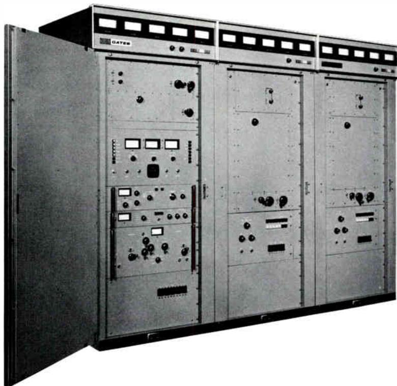
Front view, 8T-18L, 18 kW low band transmitter, showing from left to right, the 1300-watt exciter/driver, the aural power amplifier and the 18 kilowatt visual power amplifier.
