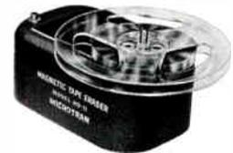
Professional model HD-11M. Heavy duty unit erases entire reel of tape at once, in seconds. Lowers residual noise 3 to 6 dB below most erase-head levels. Recommended for tape cartridges or reels up to 10½". Adaptor hub available for 10½" NAB reels. 117 volts, 50/60 Hz. Weight, 9 lbs. Made by Microtran.
