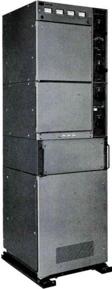
The Gates HFL-3000 linear amplifier is rated at 3000 watts CW/PEP, and is designed to operate between 2 and 30 MHz. It features continuously variable tuning over the entire range and may be excited by any suitable generating equipment delivering 100 mW of power into 50 ohms. Any type of emission not exceeding the amplifier power output or bandwidth ratings is possible.
