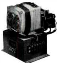
This unit for tuning variable inductor, capacitor or other controls, has built-in limit switches. Five wire reversible motor 1 rpm. Requires M-4806 relay assembly for control. 115 volt, 50/60 Hz.
