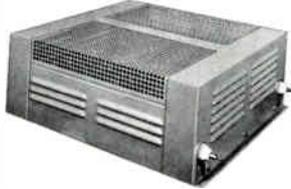
first problem is always locating the source of the trouble. An open transmission line, a short in the coupler or phasor, a short in a tower light, etc., will usually react by operating the overload relay in the transmitter. By attaching the dummy antenna, the trouble spot is quickly isolated as either in the transmitter or elsewhere in the system.
