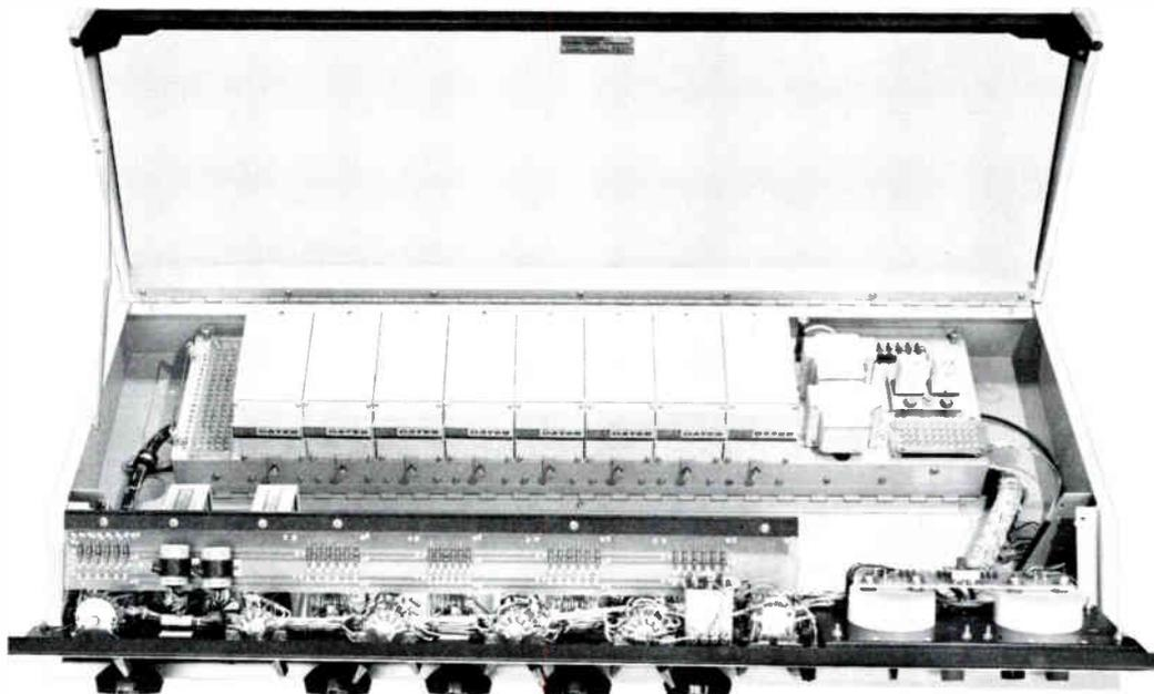
The Stereo Statesman top cover hinges up and the front panel swings down to reveal every "behind the panel" component. This layout and logical access is typical of the complete line of Gates consoles, and reflects the engineering and planning required for neat, professional installations.
