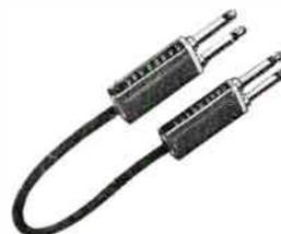
Patch cords have double plug each end, with cords in 4 lengths. Cords shielded and covered with double black braid, with extra reinforcement 6" from each plug end.
