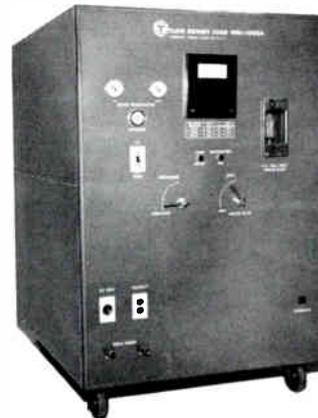
Designed for high power application, the Model WDL-1000A water cooled dummy load will dissipate a generous 100 kW AM at any frequency up to 30 MHz. Operating impedance is 300 ohms balanced. Other impedances available on special order. This model employs its own captive water system and an external heat exchanger. Water required for cooling need only be reasonably clean and free
