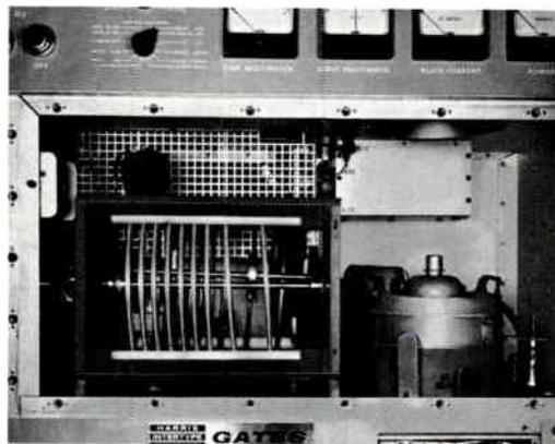
A single 8171/4CX10,000D ceramic tetrode, operating Class AB<sub>1</sub> in a grounded screen configuration, produces the full 10 kW PEP or CW output with maximum stability.
