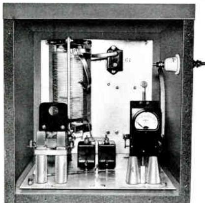
Recommended for broadcast transmitter powers of 1,000, 500 and 250 watts, 100% modulated. Heavy edgewound micaex insulated silver plated coil has generous inductance for a full Tee network along with fixed mica capacitors supplied. Extra room is provided to install either diode or thermocouple remote metering equipment. Heavy duty meter shorting switch eliminates antenna meter from the circuit when not in use for lightning protection. Meter is observed through plexi-glass porthole.
