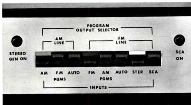
**PROGRAM OUTPUT SELECTOR:** Functions are logically presented and color-coded to channel keys and VU meter illumination for simplicity. Briefly, control provisions are: two separate transmitter inputs are marked "AM Line" and "FM Line." The AM transmitter may be programmed independently through any mixing channel when corresponding keys are operated to the left. Illuminated channel key, AM VU meter, and tab key #1 of the selector assembly are color-coded green.
