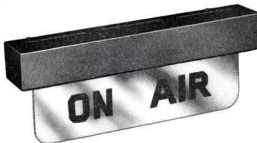
An unusually attractive studio fixture with edgewise lighting of a plexiglass transparent plate. Incandescent lamp is housed in gun-metal casing. Mounting is usually above studio door. "On Air" lettering is in red with other nomenclatures, such as Studio A", etc., supplied in black. Housing is well ventilated, without light leakage. Size: 18" wide, 3" front to back, and 6½" from bottom of glass to top of housing. 117 volts, 50 watts. UL approved.
