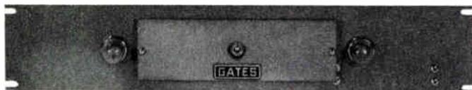
Each rack of audio and radio frequency equipment should have a master switch and fuse panel. Usually mounted at the bottom of the rack, the Gates M-4242 switch and fuse panel includes dual pilot lamps to indicate input and output voltage, dual fuses and D.P.D.T. primary switch. Rating 15 amperes at 115 volts, AC. Size: 19" x 3½" x 3" deep. Finish: Beige-gray. Weight packed: 10 lbs. Cubage: 1 cubic foot.
