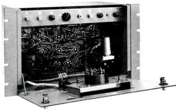
Front panel hinges down for easy maintenance and operating adjustments. Note the circular temperature-controlled oven containing all oscillator components and the precision vacuum type crystal. A slip-on dust cover protects tubes and terminations.
