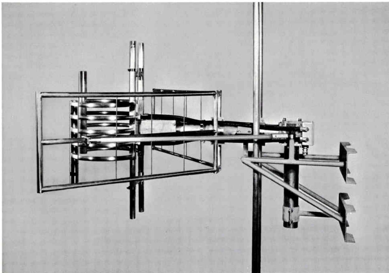
Gates' FMC-(X)DA is a directional dual polarized FM antenna designed for pole mounting. The antenna is available with up to eight bays (the X in the type number indicates the number of bays—the 4-bay antenna is FMC-4DA, etc.). The interbay transmission feed line uses  $3\frac{1}{8}$ -inch rigid coaxial line. Spacing between bays is one wavelength.
