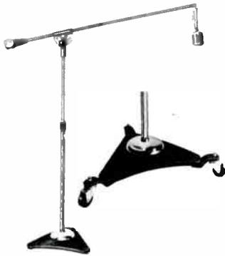
Provide convenient and proper microphone placement where correct position cannot be reached with conventional stands. Boom length 62 inches, height adjustable from 4 ft to 6 ft. Base diameter 17 inches, tubular sections super-chrome plated. "Snap On" hangers provided for microphone cable. Shipping weight 33 lbs.
