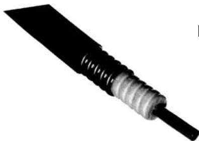
Foam Heliax is used in those broadcast installations requiring low loss coaxial cable in which pressurizing is not desirable. A corrugated copper outer conductor and foam dielectric provide a combination of high strength, low loss and power handling not available in solid dielectric cables. The flexibility of foam Heliax provides maximum resistance to crushing, kinking or denting, and enables it to be pulled through conduits and around obstructions. Please order by type number.
