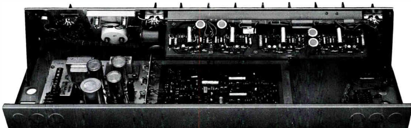
Complete access to all components is via the easily removed cover of the Yard II. All input and output connections can be made through the rear or the bottom of the console. Convenient knock-outs on the rear apron provide entry for wiring cables.
