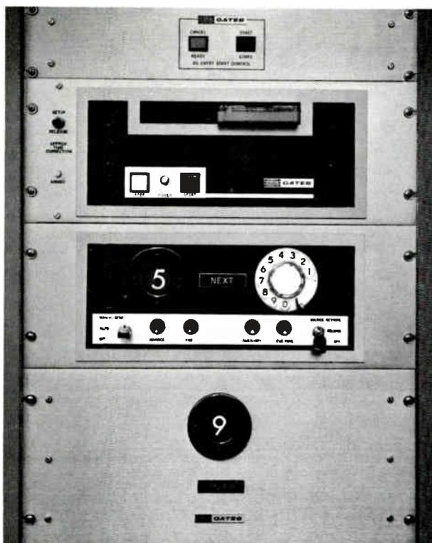
The SP-10 and SP-19 program control systems provide fully automatic control of audio automation systems. The SP-10 unit will function with up to 10 audio sources, and as many as 19 may be controlled with the SP-19 Programmer.
