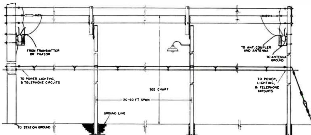
Chart above illustrates typical five or six wire open type transmission line. Table is provided to show impedances with various wire sizes at certain heights above ground. Transmission line brackets are M-3327, end plate M-3328. Horn gap is M-3322. The power, lighting and telephone circuits shown are optional, according to requirements of installation.
