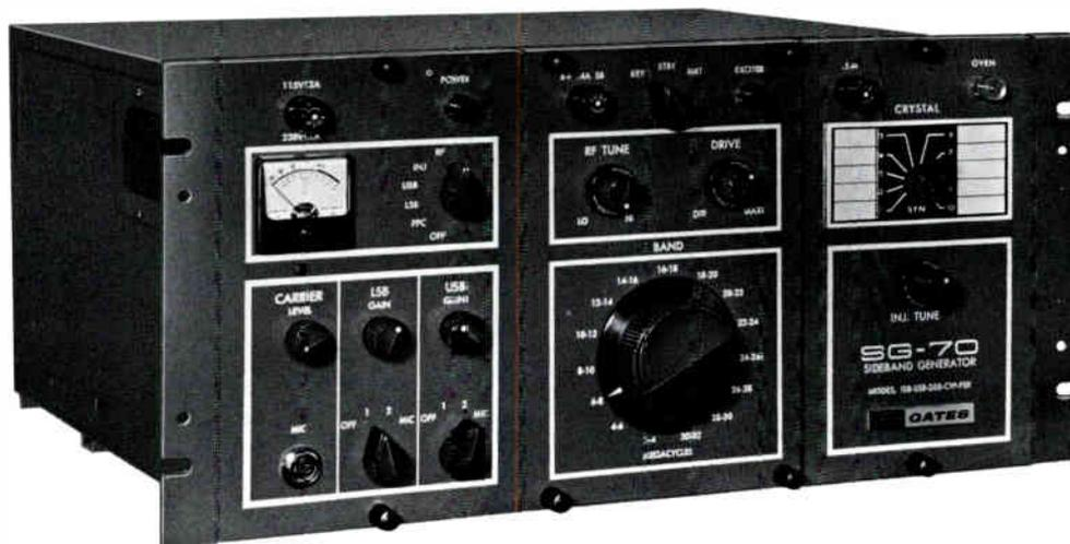
Gates Model SG-70 ISB exciter is equipped to transmit single sideband, independent sideband, compatible AM, CW, MCW, or FSK with adapter. Provisions are incorporated for carrier suppression from  $-50$  dB to  $0$  dB. A versatile and compact unit designed for accurate and rapid channel change and tune-up, the SG-70 has a self-contained silicon rectifier power supply, and requires only  $8\frac{3}{4}$  inches in a standard 19-inch rack for mounting.
