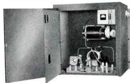
Housed in aluminum cabinet with double front doors. Porthole for meter reading and heavy duty meter shorting switch operates with doors closed. Large micaex insulated silver plated coils combined with capacitors of generous voltage and current ratings to assure a lifetime of service under extreme heat or cold. A large antenna lead in bowl is provided. Mounting is with metal flanges on the back of the tuning unit for attachment to wooden poles set in ground or for mounting on wall.
