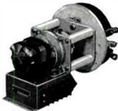
Recommended for regulating the plate voltage in transmitters of 1 kW and less. Available in three sizes for 250, 500 and 1000 watt transmitters. Motor is one rpm and operates from 115 volts, 60 Hz.
