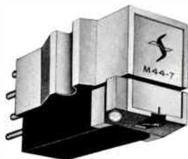
Model M44-7 stereo dynetic cartridge is recommended for faithful reproduction of both stereophonic and monophonic recordings. It offers superior stereo separation, smoother response, and is designed to complement the 15° effective cutting angle now being used on stereo recordings. The easily changed styli may be interchanged for various types of recordings.
