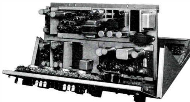
The Studioette top cover may be completely removed, and the front panel hinges out to reach every "behind the panel" component. The amplifier deck hinges up so that muting relay contacts are at your finger tips when touch-up burnishing is required.
