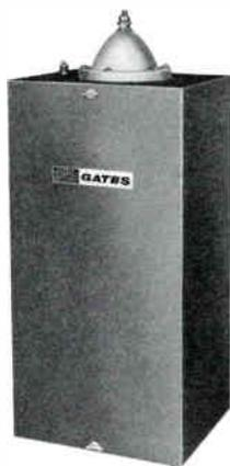
Both series and shunt fed models are constructed in a non-weatherproof cabinet with slip-off front door and large lead in bowl at top. Coil is micaex insulated edgewound silver plated and capacitors are supplied to tune to buyer's specific frequency. Size: 21" high, 10" wide, 9" deep. Usually mounted in small dog house at base of tower. Rating 1250 watts, 100% modulated.
