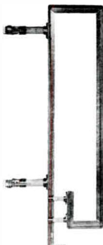
This is a very rugged fixed non-shielded RF sampling loop. It is heavily galvanized after welding, and is fitted with large steatite insulators and heavy duty tower leg clamps for easy and positive mounting. Complete with type "N" jack. For 50 to 70 ohm sampling line.
