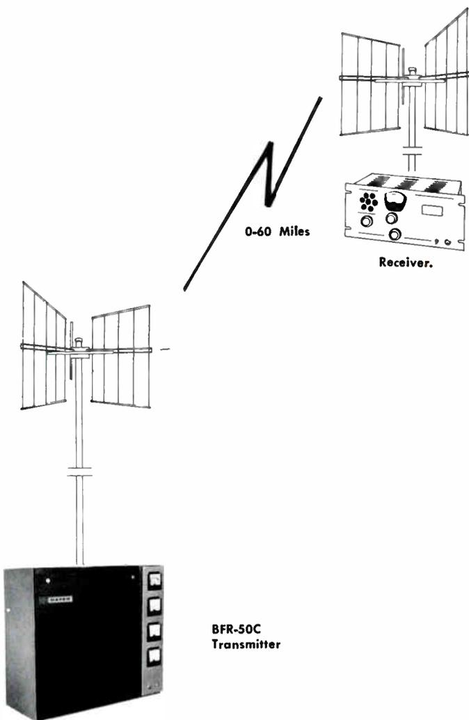
**DIRECTIONAL:** System A is a directional FM system operating in the 148-174 MHz band, which furnishes an effective 750 watts signal and will provide a line-of-sight high fidelity transmission link over distances up to 50 to 60 miles (subject to antenna heights and terrain). Applications include studio to transmitter link, point to point relay service, or remote pickup. Featured is the Gates BFR-50C, 50 watt Transmitter.
