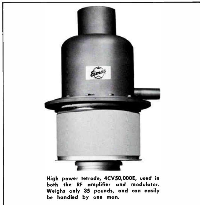
High power tetrode, 4CV50,000E, used in both the RF amplifier and modulator. Weighs only 35 pounds, and can easily be handled by one man.
