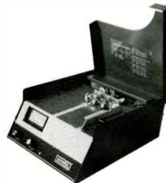
The hinged top cover of the CD-15 provides immediate access to the head mount and cartridge engage lever. Input and output terminals are located on the rear panel. The cabinet housing and transport deck are of heavy gauge steel with a baked enamel finish. A precision VU meter is mounted in the front panel.
