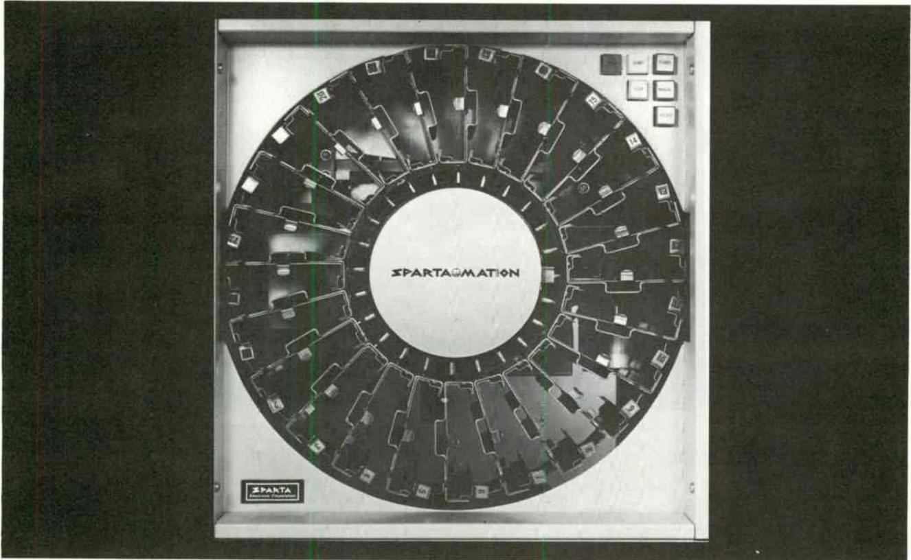
Spartamation RS-124 monaural and RS-224 stereo Carousels are the ultimate in multi-cartridge reproducers. They feature a 24 cartridge capacity, all plug-in solid state logic, new tray design, teletype logger output, and random selection.
