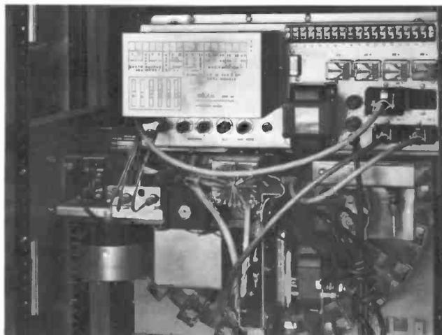
The Carousel is mounted on brackets which connect to the front and rear vertical rails of Sparta CAB-61 racks. The entire electronic section can be disconnected and removed in 2 minutes. All active circuits are on plug-in printed circuit boards.
