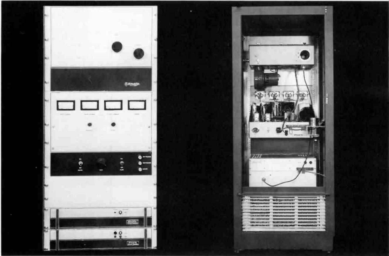
Sparta's Model 600A FM Transmitter for standby or low power operation offers the buyer a choice of space saving cabinet housings. All components of the Model 600A are a standard 19" rack size and due to their compactness can be consolidated into a single rack with monitors, remote control and STL equipment.
