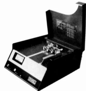
The hinged top cover of the CD-15 provides immediate access to the head mount and cartridge engage lever. Input and output terminals are located on the rear panel. The cabinet housing and transport deck are of heavy gauge steel with a baked enamel finish. A precision VU meter is mounted in the front panel.
