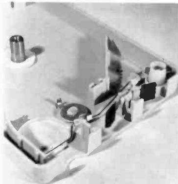
*The Model 350 is a modification of the standard Fidelipac Professional Cartridge. It includes a Corner Post which uses a cross-arm to guide the tape vertically. Turning the adjusting screw raises or lowers the arm as required. Access to the screw is through a hole in the cartridge cover.*
