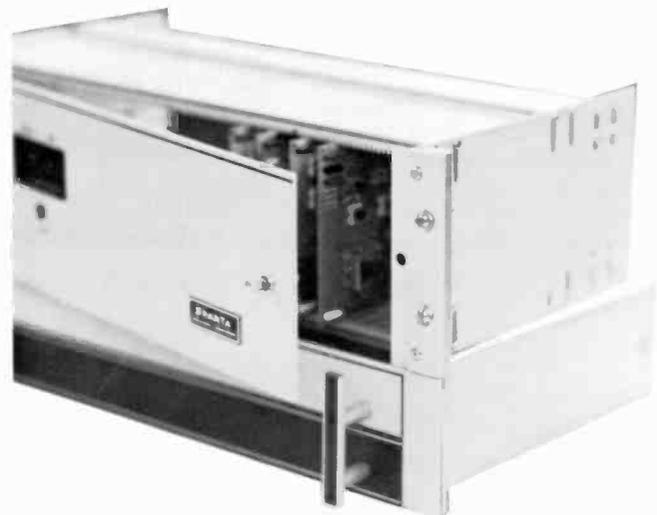
One RS250 and two RS124 Carousels are most commonly supplied with interconnecting cables cut for mounting the Random Access directly above adjacent Carousels. This combination, unmounted, is available as the SPARTAMATE "SPOT BANK" package for addition to existing SPARTAMATION or other automation systems. The RS250 takes 8 $\frac{3}{4}$ " of rack space.
