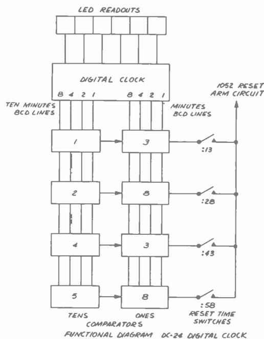
*Digital Clock with thumbwheel switches for control of automatic network joining.*
