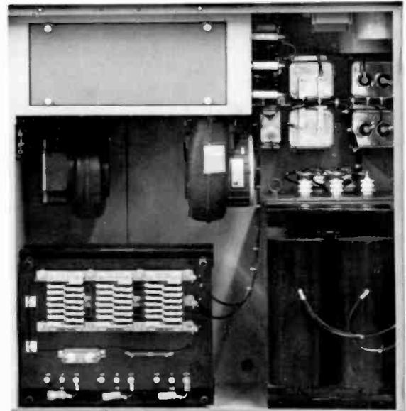
The outward appearance of both the Model 705 and 710 AM Transmitters is very similar. The metering and control functions in the 705 and 710 are identical. The difference is shown directly above. The power supply, modulation transformer and reactor are larger in the 710.
