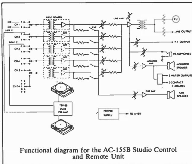
Functional diagram for the AC-155B Studio Control and Remote Unit
