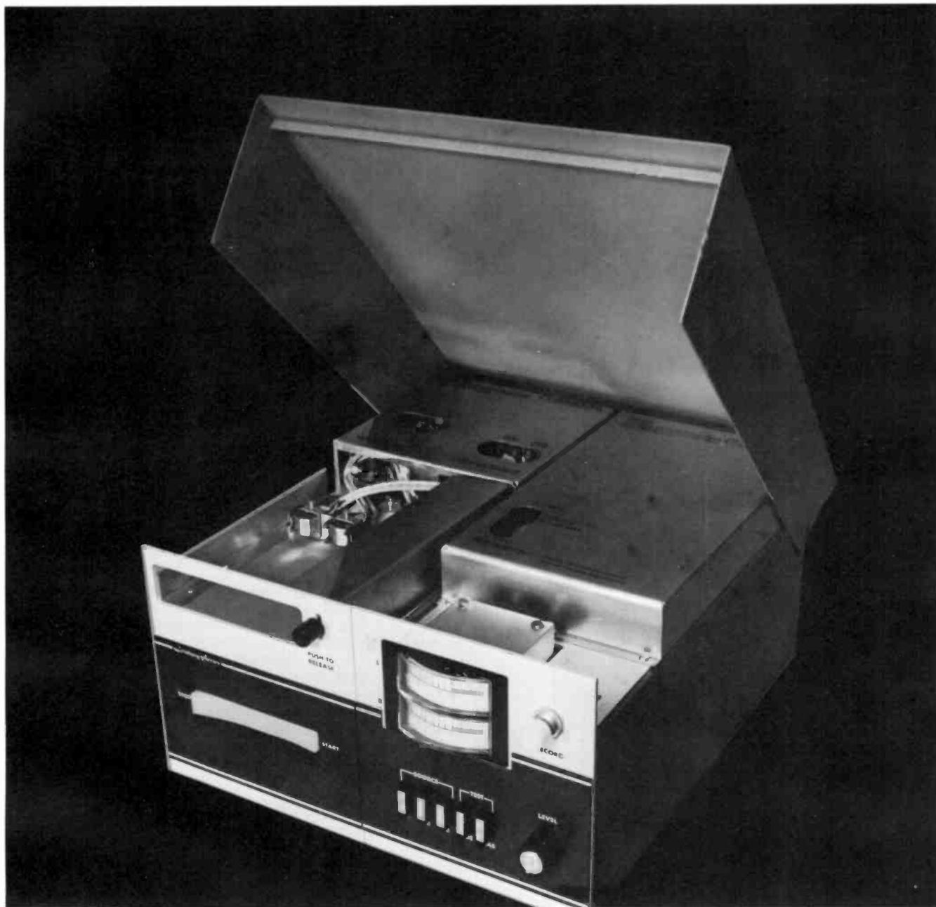
The CENTURY SERIES by SPARTA is a modular line of tape cartridge equipment uniquely styled and engineered to set new standards of excellence. The compactness of the modules enables three to be mounted side-by-side in standard rack cabinets. There are also single, dual, and 'quad' housings for table-top use. The entire Record/Playback system occupies only 1 1/2x15" of desk space, and stands a
