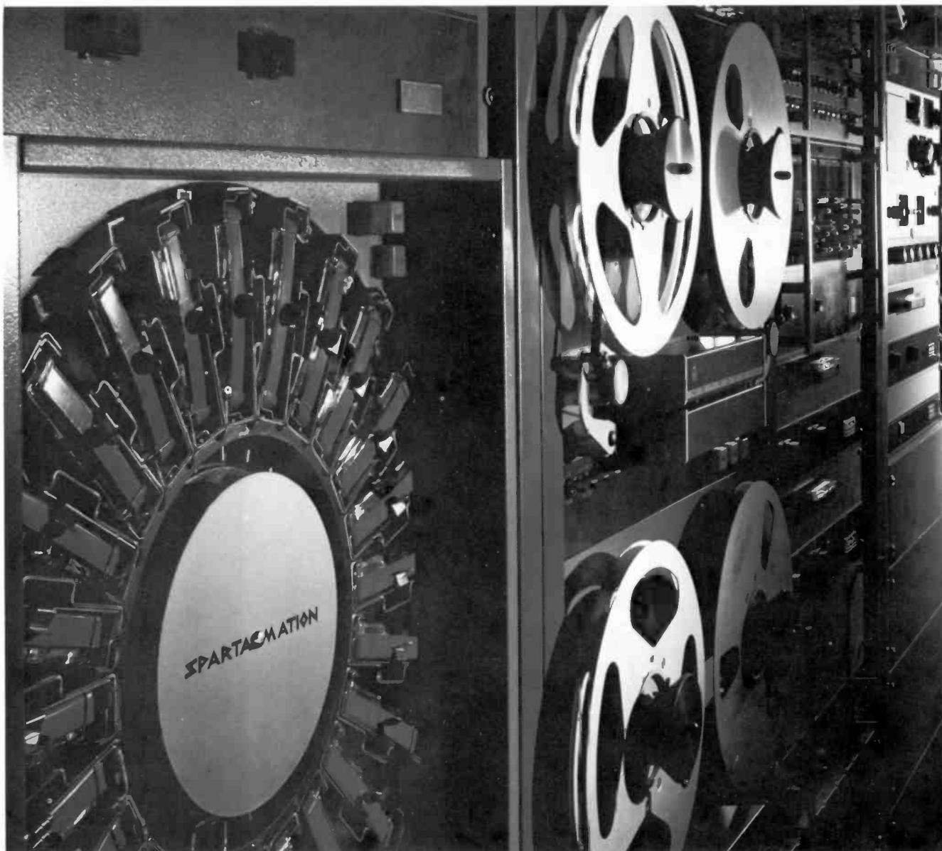
It really isn't as complicated as it looks! A Spartamation system consists mostly of audio tape reproducers. Usually they're multi-cartridge types for commercials, and either reel or multi-cartridge reproducers for music. One or more single cartridge playbacks are used for ID's and repetitive format material. A cartridge Random Access can be added—a series of 24 position slider switches to select the order in which commercial cartridges will play.
