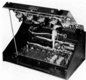
Front panel lifts for easy access to individual circuit modules. A convenient quarter-turn fastener securely locks the panel in place.
