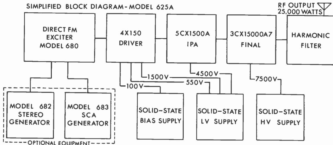
Model 610A: RF output 13,000 watts. LV supply to IPA 2600V. HV supply to final 5600V. Final tube is 3CX10000A7. All other details of block diagram are identical to Model 625A.
