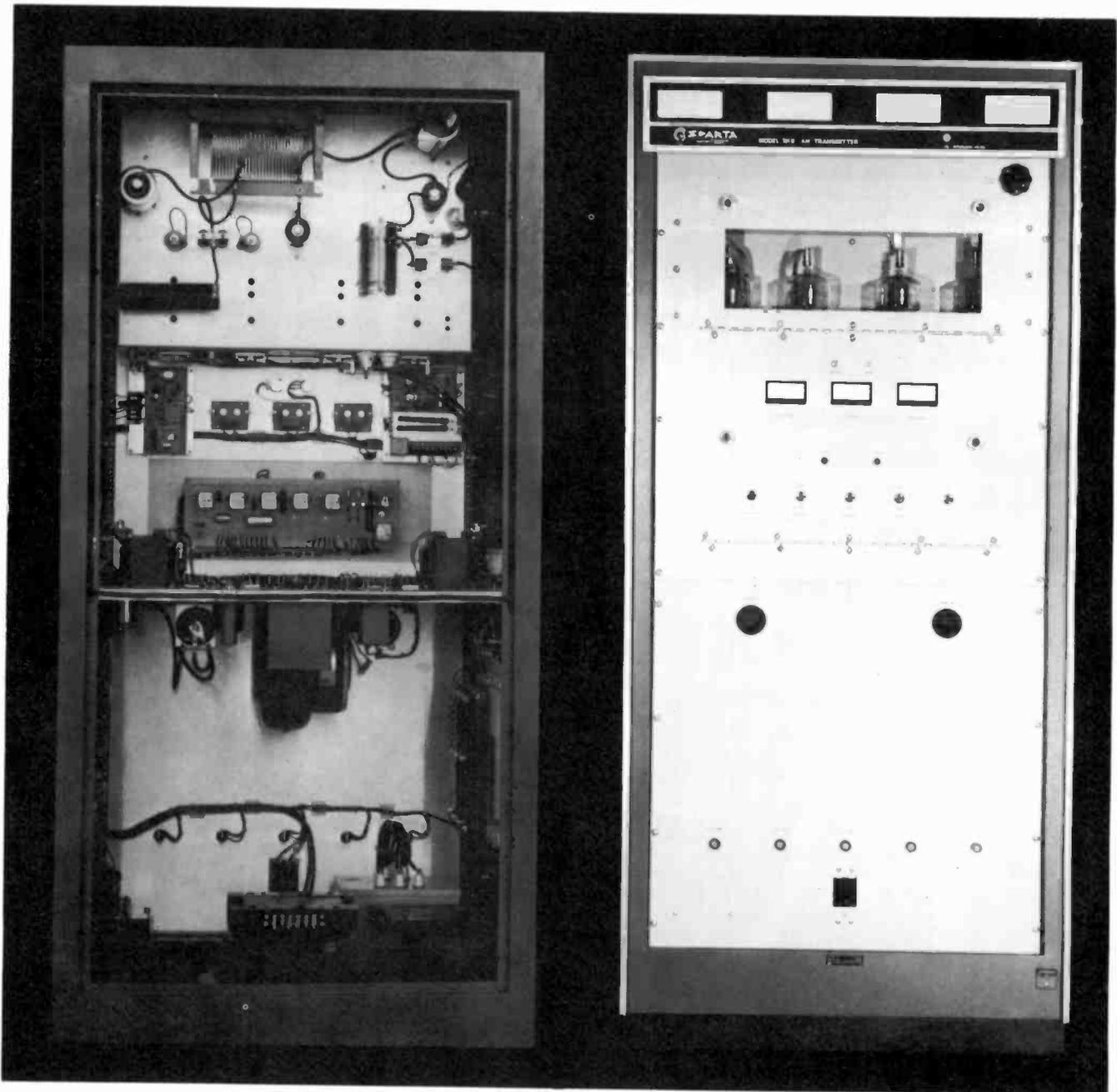
The simple straightforward engineering design of the new Model 701B is illustrated even in the classically simple layout of the front panel. The panel below the tubes and meters drops down for easy access. On its face are the "tally lights," which tell the engineer at a glance where his overload problem may have occurred, even though the automatic reset has returned the transmitter to the air.
