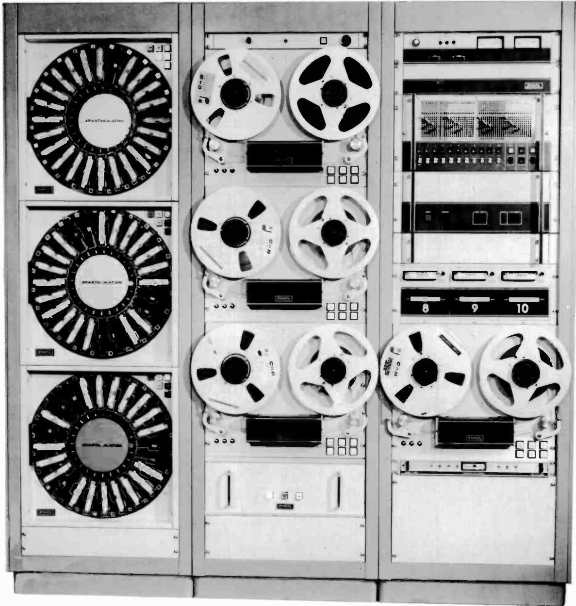
**COMMERCIALS:** RS-124 or 224 Carousels™ assure quality playback of stereo or mono announcements. Each Carousel holds 24 cartridges. Each cartridge can hold several spots that play in rotation — up to 10½ minutes per cartridge. Each time a cartridge is played, the next announcement is read by the Cartridge Random Access.
