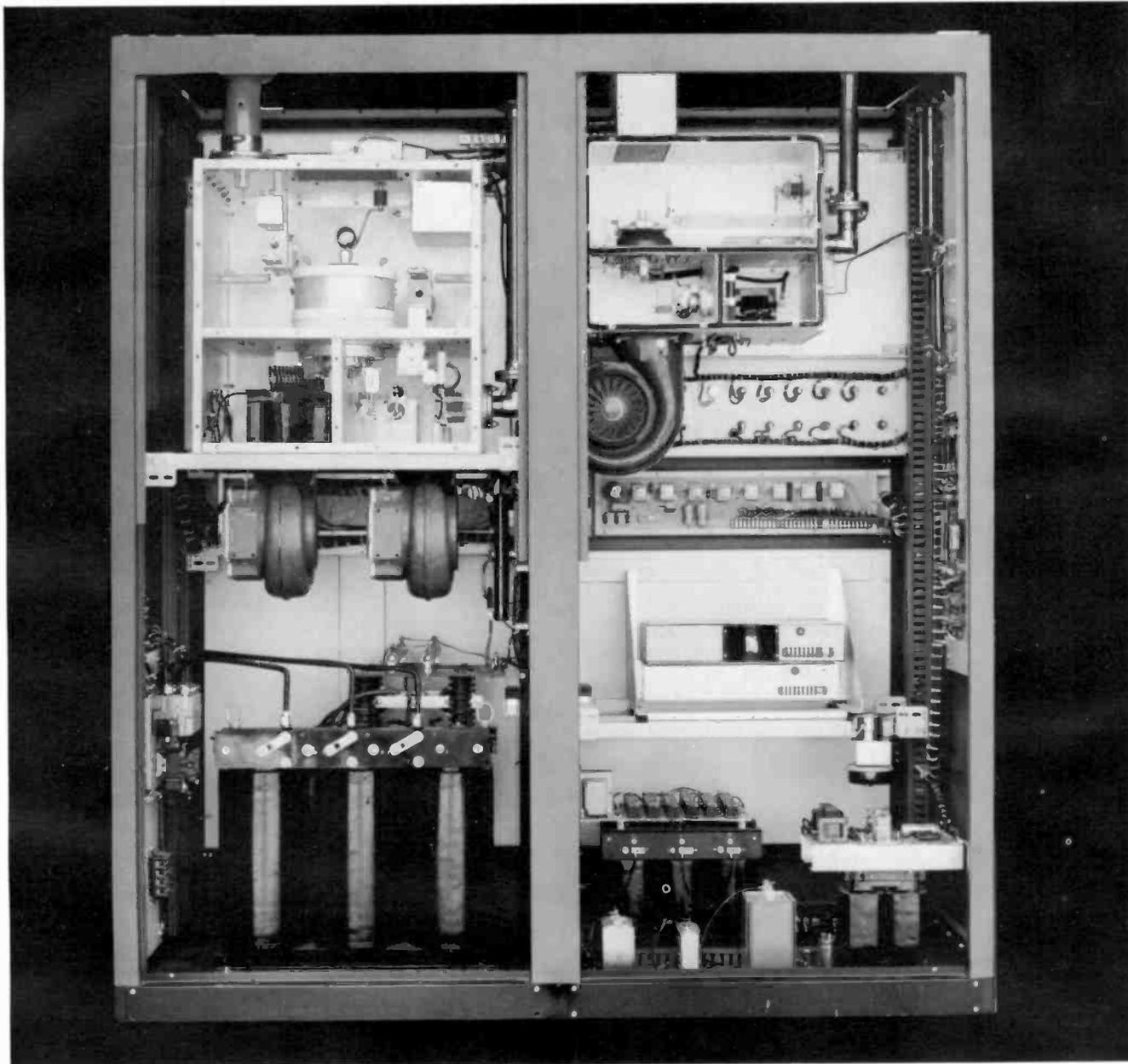
The above picture shows the roll-out high voltage power supply which is contained within the main transmitter housing. There are four heavy-duty "dolly" type casters upon which the power supply
