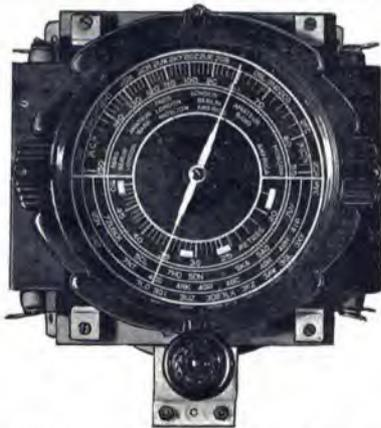
SCALES—“Edgelit” Glass either D/W or B/C only. Fully calibrated on both bands.
