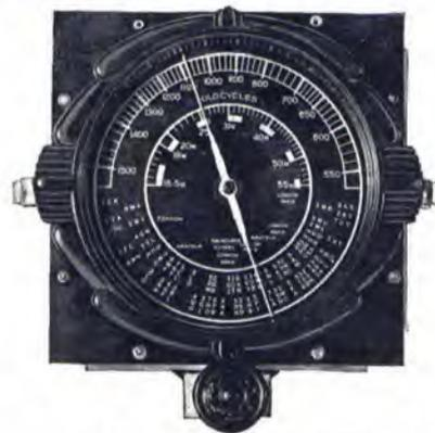
This model has met with great approval, due to its adaptability to any chassis. It was designed to permit the gang to mount directly on to the chassis, without the necessity of cutting a wide hole in the chassis, or alternatively mounting the gang on brackets or spacers as is required with the FD7, FD7G and FD8G dials.
