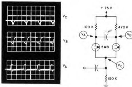
Fig. 3.25. Typical Monostable Multivibrator Operation.
