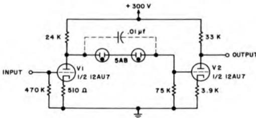
Fig. 4.9. Glow Lamp Coupled Amplifier.
