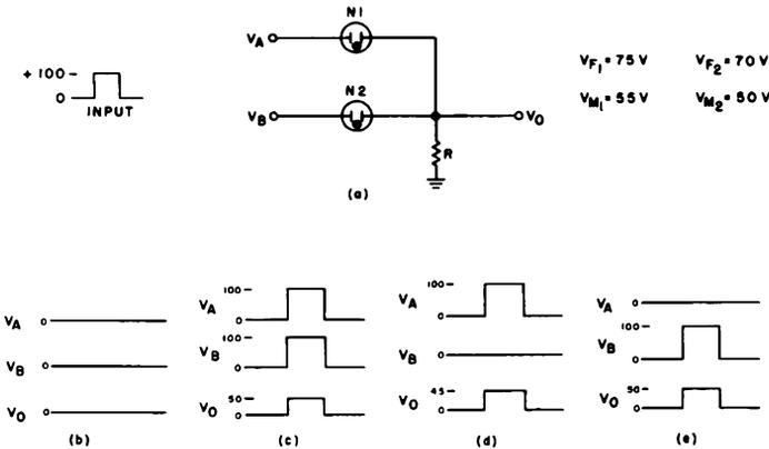
Fig. 3.10. Waveforms for Basic 2-Input "OR" Gate.
