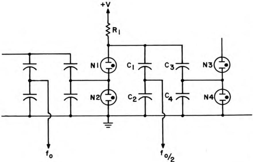
Fig. 2.26. Basic Configuration of Frequency Dividing Tone Generator.
