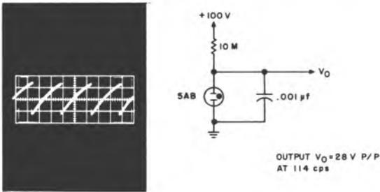
Fig. 2.12. Typical Sawtooth Oscillator Low Frequency Output.
