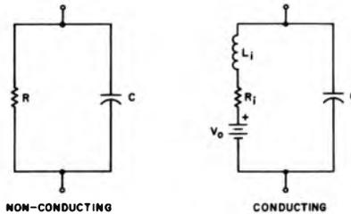
Fig. 1.4. Equivalent Circuits for the Glow Lamp
