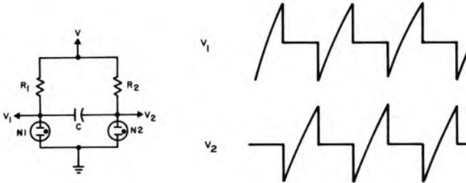
Fig. 2.19. Typical Glow Lamp Astable Multivibrator and Outputs.
