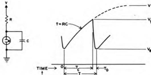
Fig. 2.2. Single Cycle of Typical Sawtooth Output
