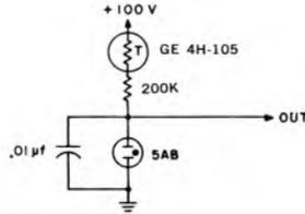
Fig. 2.33. Temperature Indicator.
