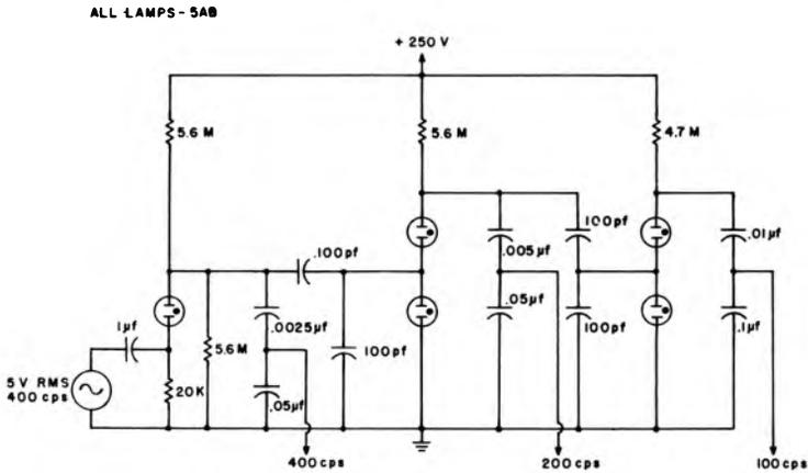
Fig. 2.27. Typical Frequency Dividing Chain.
