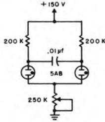
Fig. 2.22. Glow Lamp Multivibrator with Common Cathode Resistance.
