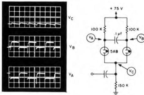
Fig. 3.24. Typical Bistable Multivibrator Operation.
