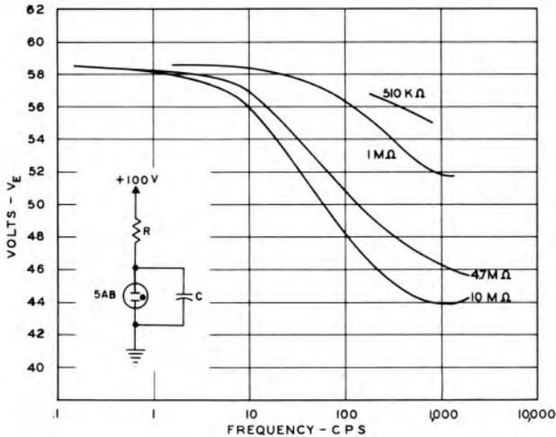
Fig. 2.16. Variation of Extinguishing Voltage - Constant Resistance.
