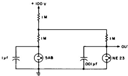
Fig. 2.31. Glow Lamp Audio Alarm Circuit.
