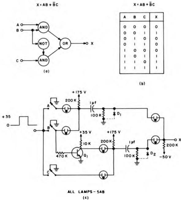
Fig. 3.15. Glow Lamp Logic Circuit (AC Coupled).
