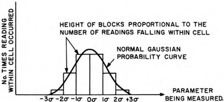
Fig. 5.8. Arrangement of the data in histogram form.
