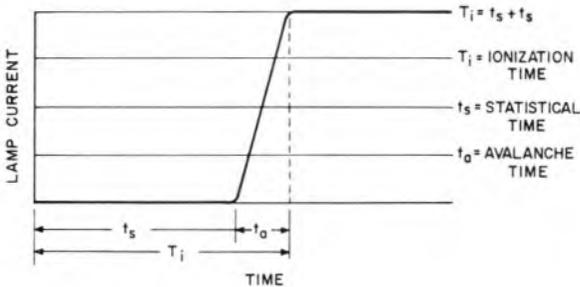
Fig. 5.6. Delay times for neon turn-on defined.
