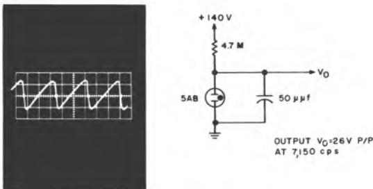
Fig. 2.13. Typical Sawtooth Oscillator High Frequency Output.
