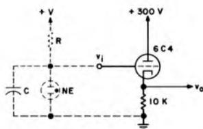
Fig. 5.3. Test Circuit for Determining Dynamic Lamp Characteristics with Lamp Circuit Isolated from Output.
