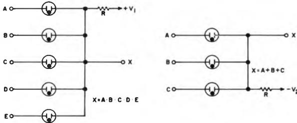
Fig. 3.16. "AND" and "OR" Gates with Multiple Inputs.
