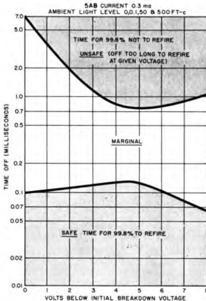
Fig. 5.12. Time-off as a function of refiring voltage.
