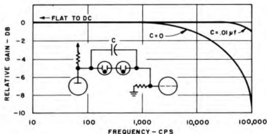
Fig. 4.10. Amplitude Response of Glow Lamp Coupled Amplifier.
