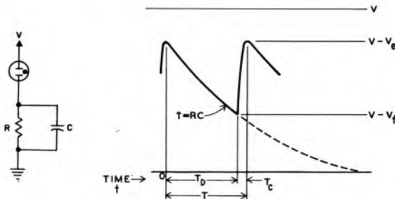
Fig. 2.3. Single Cycle of Typical Sawtooth Output
