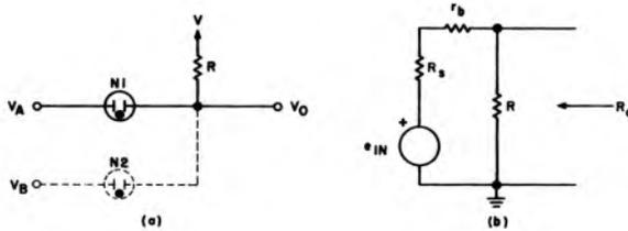
Fig. 3.8. Equivalent Circuit of Glow Lamp "AND" Gate.
