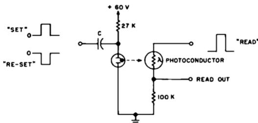
Fig. 3.29. Glow Lamp — Photoconductor Memory Circuit.
