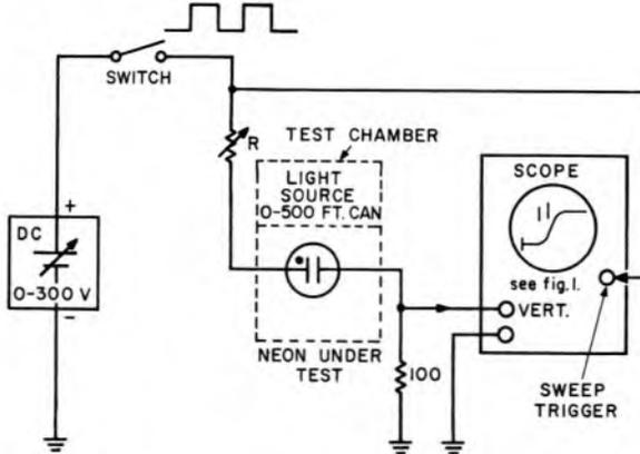
Fig. 5.7. Setup for measuring a neon's ionization time.
