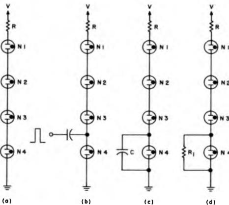
Fig. 4.4. Starting Methods for Glow Lamp Regulators.
