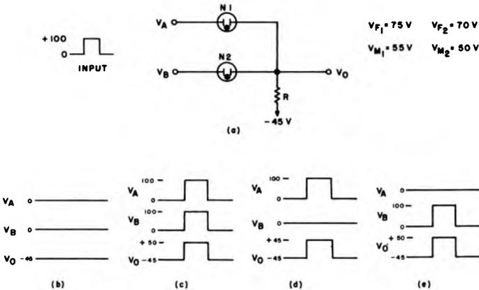
Fig. 3.12. Waveforms for Modified 2-Input "OR" Gate.
