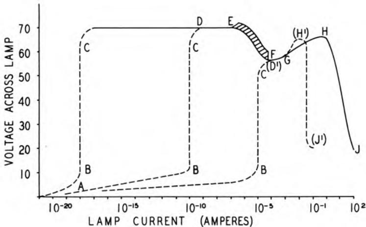
Fig. 1.1. Characteristic Curve of the Neon Lamp
