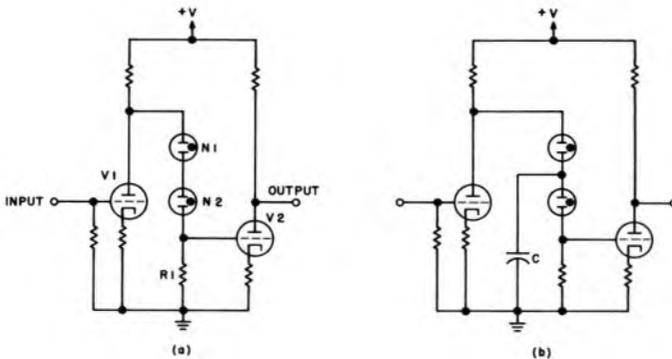
Fig. 4.7. Direct Coupled Circuits Employing Glow Lamps.
