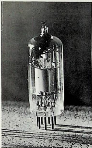
Fig. 31. The diode A.F. pentode DAF 91.
