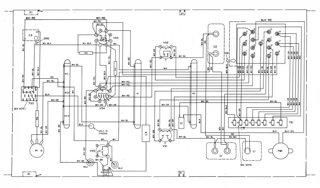
NOTE: I. IN SOME EQUIPMENTS, STRAPS WILL BE FOUND CONNECTING TERMINALS 6 & 7 AND 9 & 10. THESE MUST BE REMOVED BEFORE POWER IS APPLIED TO APPARATUS.
