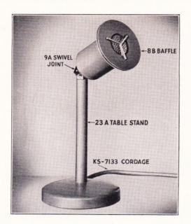
angle. The 9A Swivel Joint is available for this purpose. The directional effect may be further accentuated by the use of the 8B Baffle, a disc 3-1/4" in diameter which fits snugly over the face of the microphone and increases its sensitivity for sounds arriving at 0° over the range from 1000 to 5000 cycles. This feature is useful in helping speech sounds override surrounding noises.
