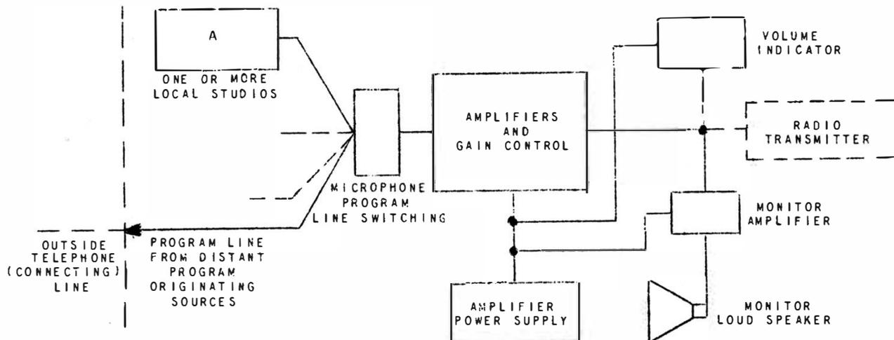
Many smaller broadcasting systems have entered into contractual relations with one or more larger stations which provide program networks for this type of service. The program thus received is amplified locally and broadcast in a manner similar to that employed with a program originating in the station's own studios.
