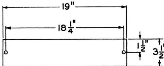
GENERAL Primarily designed for the 1219A Panel which is a part of the 9A Speech Input Equipment. Provides a mounting for the terminal strips for the incoming and outgoing speech circuits
