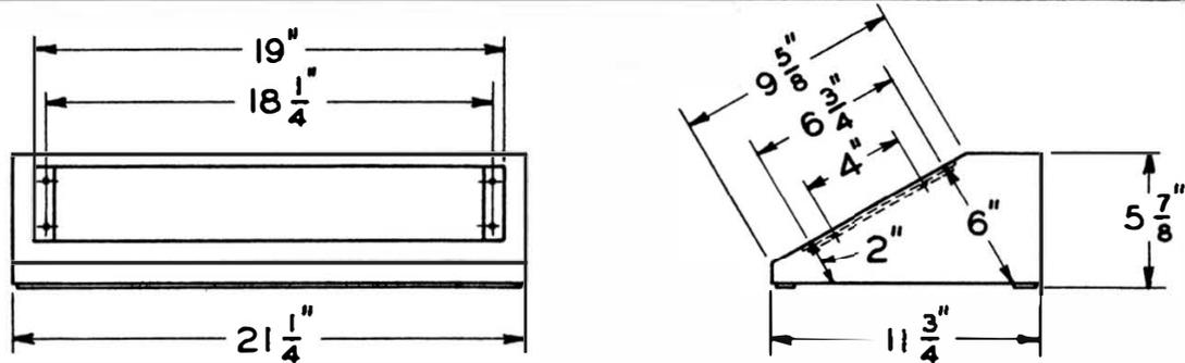
**GENERAL** Designed primarily to mount a 267A Control Panel for table or desk use in Speech Input Equipment assemblies.
