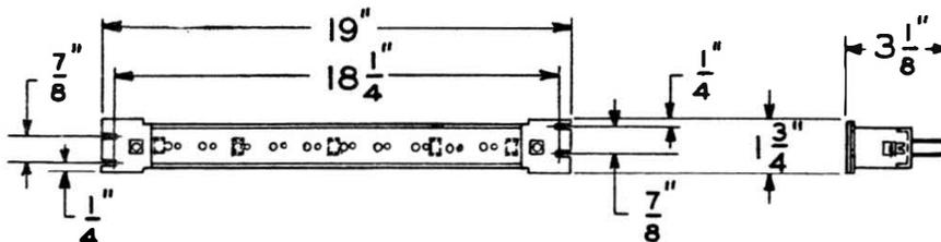
GENERAL Designed primarily for Speech Input Equipment assemblies for mounting a total of ten 700A Terminal Strips or 11A Connecting Blocks.
