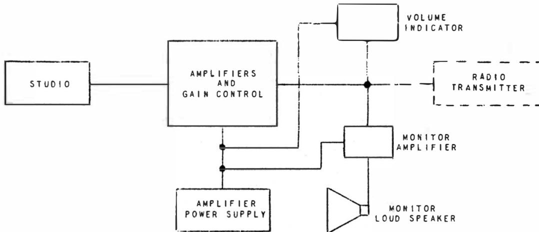
Since the studio and the radio transmitter are so closely associated, telephone lines are not needed for program transmission and only a minimum of speech input equipment is required. This usually is of the single channel type, that is, only one amplifier system with the necessary amplification and control to accommodate one program at a time.
