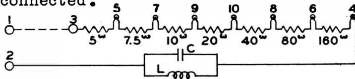
Non-loaded cable circuits consisting entirely of one gauge can be equalized up to the approximate lengths given below by the use of the 23A Equalizer.
