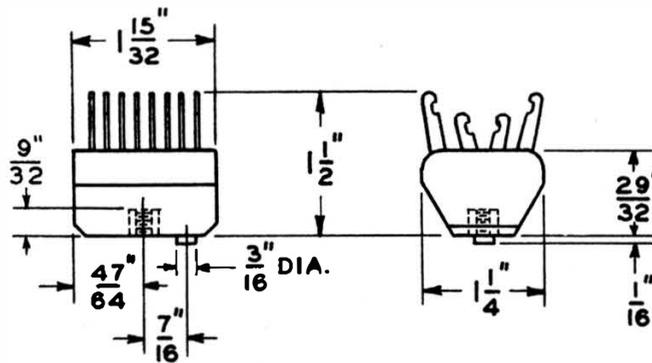
**GENERAL** Improved type of terminal strip intended primarily for Speech Input Equipment panels and assemblies.
