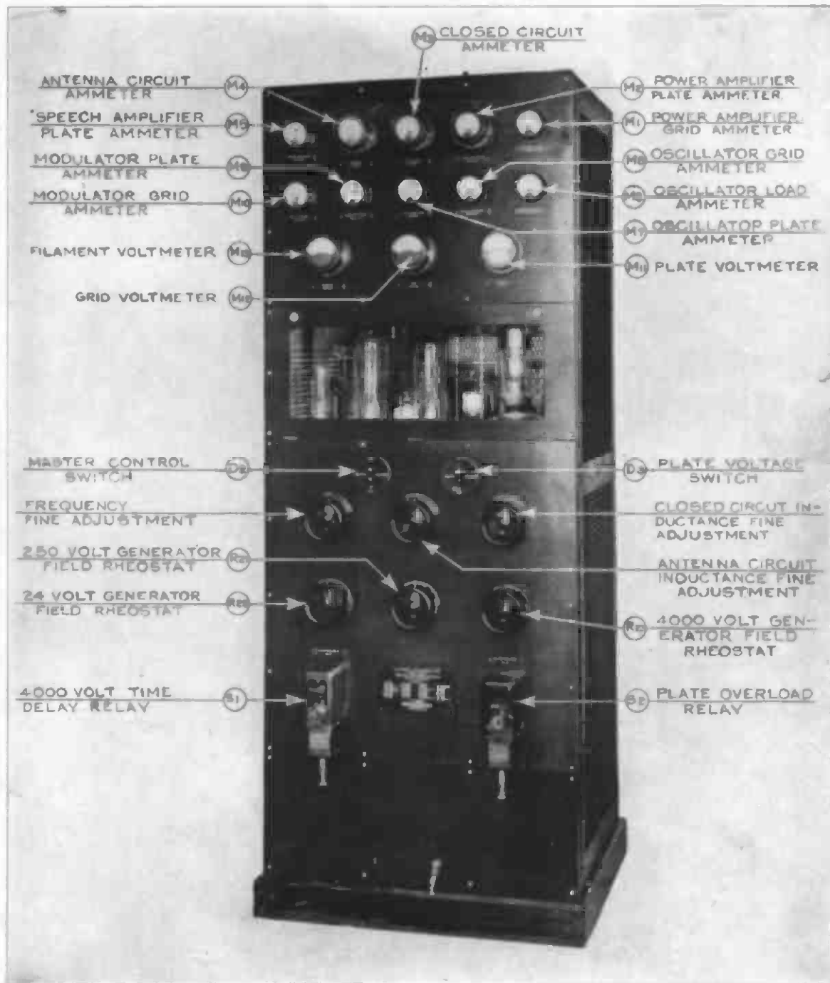
6-A RADIO TRANSMITTER FRONT VIEW—25453
