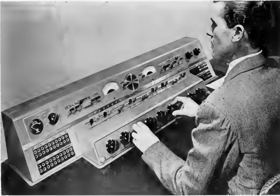
Operator at 40A Console mounted in KS-10284 Table. Controls are grouped functionally with frequently used controls nearest operator and all controls within convenient reach. Low over-all height and location of console contribute to increased operator efficiency and reduced operating strain. Over-all height is 3 feet from floor and 8½ inches from writing surface. Over-all length of table is 54½ inches and control panel 48 inches. From front to rear it is 28½ inches and from control panel to rear 13½ inches.
