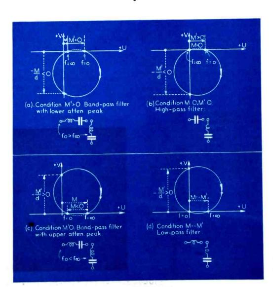
THIS paper describes how a picture of the behavior of wave filters may be obtained by the use of simple graphical methods.
