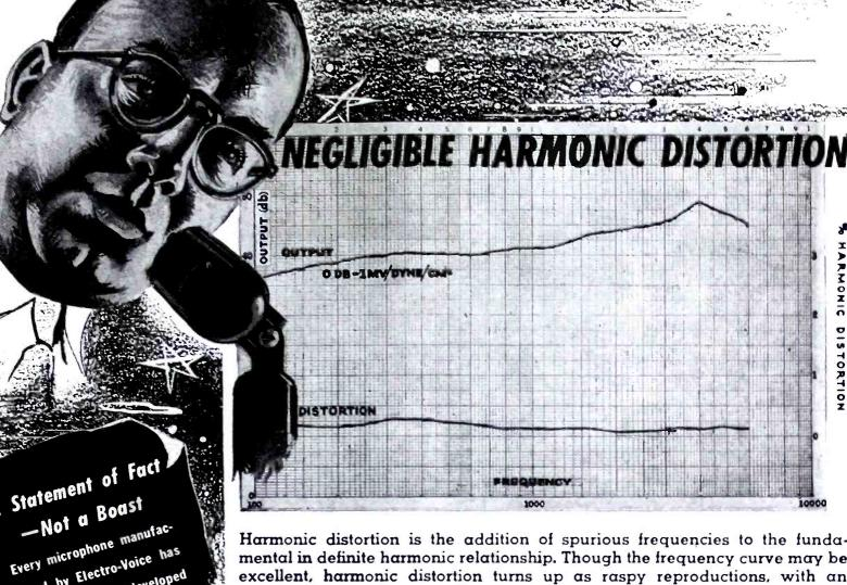
Harmonic distortion is the addition of spurious frequencies to the fundamental in definite harmonic relationship. Though the frequency curve may be excellent, harmonic distortion turns up as raspy reproductions, with an unnatural twang, in microphones, amplifiers and speakers. Five percent is considered a satisfactory upper limit for good reproduction, and as much as fifteen percent is allowable for speech communication.
