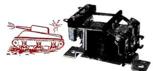
SERIES 165 VIBRATION RESISTANT Counterbalanced armature and sturdy construction throughout give this relayan unusual resistance to vibration. Silver contacts are rated at 12½ amperes in combinations up to double pole, double throw.
