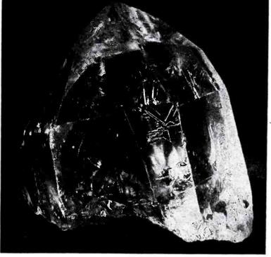
Portion of large prismatic crystal, showing cracks, chips, optical and electrical twinning surface patterns.
