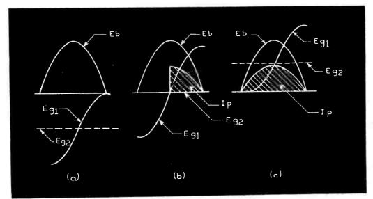
grid voltage d-c component, which is variable in magnitude and is reversible in polarity with respect to thyratron cathodes. This follows, since the cathodes of the thyratrons are connected with the voltage divider center tap, the latter being connected across the separate control d-c power supply. This is also true of the control potentiometer. The variable contact of the control potentiometer thus varies the d-c voltage and polarity of the thyratron control grids with respect to the cathodes.
