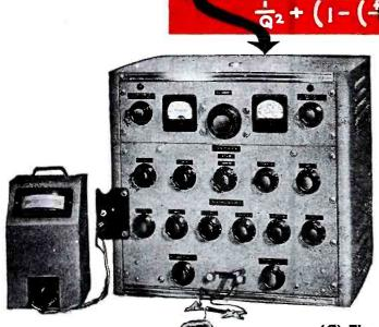
(B) The UTC inductance bridge is capable of four digit accuracy and covers a range from extremely low values to over 100 Hys. The effective resistance and inductance values are direct reading, eliminating the possibility of error in conversion.
