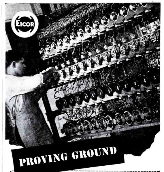
A fter a motor or dynamotor has been properly designed, built, and inspected — what then? At *Eicor* it is installed on one of these run-in lines for a series of tests extending over many hours, to subject the unit to conditions more severe than those encountered in its operating life.
