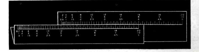
Scale A (RSS scale) arranged in typical slide rule fashion to show its use. In this particular figure, the scales are placed to show how the length of the hypotenuse of a right triangle having legs of three and four units may be obtained.
