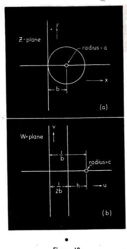
Figure 19 In *a* we have a concentric line with small inner conductor. In *b* is a single wire near ground substituted for *a* by means of the conformal transformation w = 1/z.
