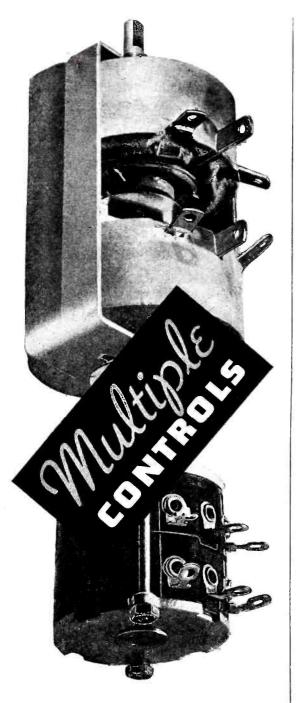
★ Another control problem — the kind Clarostat engineers like — came in recently. Specifically: a tandem assembly comprising dual 50-watt power rheostats and dual 3-watt wire-wound potentiometers; the latter insulated from shaft and ground for 2000-volt breakdown test; four units to have the same degree of rotation. In a hurry, of course; first a sample; then production running into large figures.
