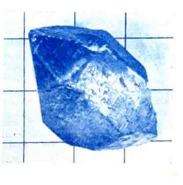
Full double-ended crystals of regular prismatic quartz, showing an apex at each end. Crystal at left shows surface inclusions. Doubleended crystals are rare because quartz prospectors generally break the crystal when chopping it away from the bed.
