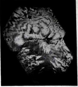
Double quartz crystal intergrowth viewed between crossed polarizers in oil bath. The line of sight of the camera is approximately parallel to the optical axis of the upper crystal. Optical twinning permeates this pair of crystals.
