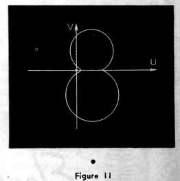
Filter path of a confluent filter. If all the points like L and H (Figure 10) are joined together, the *filter path* is obtained. This is not circular, but approximates the two circles joined together by a chord.
