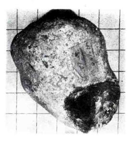
River quartz, showing the results of erosion of prismatic quartz lying in river bed for many centuries. This type of quartz is often of excellent quality because the surface imperfections have been eroded away.
