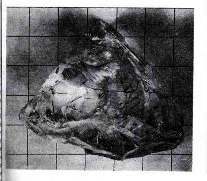
Irregular quartz. The quartz when broken shows surfaces of conchoidal fracture along poorly defined cleavage planes.
