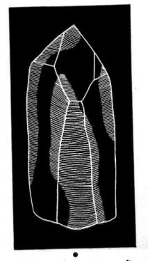
Electrically twinned raw quartz after sand blasting and etching. Shaded portions are electrical twin areas.
