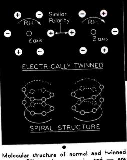
Molecular structure of normal and twinned quartz. Silicon atoms are +, and — are two oxygen atoms SiO<sub>2</sub>.
