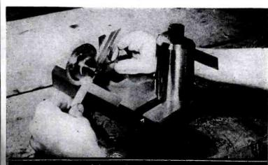
The universal bevel protractor can also be used for testing and checking various angles on finished work and work still in process.
