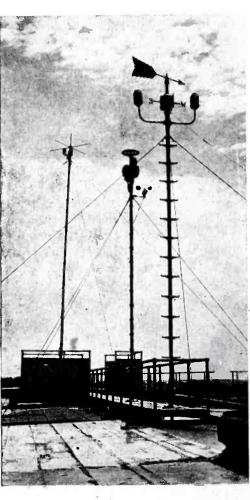
A v-h-f antenna and wind recording instrument located on top of an AACS airdrome control tower.
