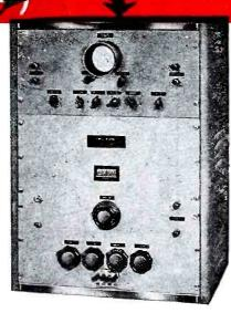
(C) The UTC oscillator is direct reading, where the frequency desired is set as in a four digit decade box, and is accurate within 1 cycle at 1.000 cycles. The range is 10 cycles to 100 kc. Accuracy of this type is essential with filters having sharp attenuation characteristics. This instrument is augmented by a UTC harmonic analyzer for the output measuring device.
