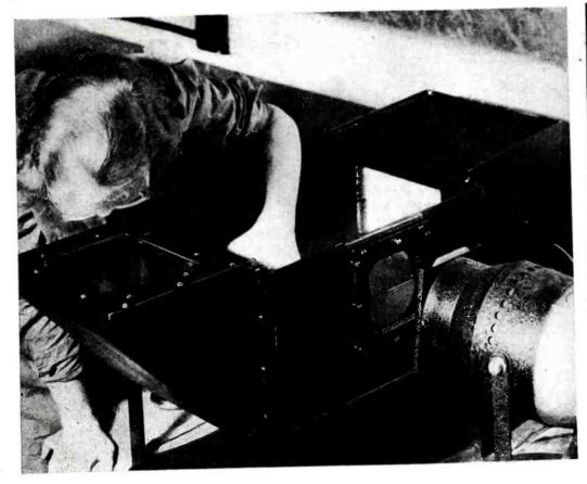
Raw quartz inspection tank having plane polarized light source with crossed polarizer as analyzer, plus high luminosity spotlight.
