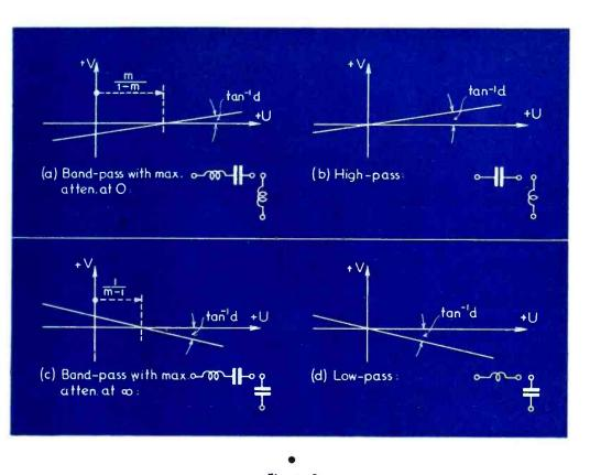
Figure 3 Filter paths of "prototypes". The circles in this case degenerate into straight lines.
