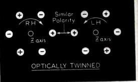
can usually observe the depth of penetration of the optical twinning and approximate its extent in terms of percentage of total volume. Electrical twinning cannot be detected this easily. Since the optical properties of electrical twinning in a quartz crystal are similar to those of the main body of the quartz, polarized light is unchanged on crossing the twinning boundary and we see no abnormal effect. We must use other means for its detection.
