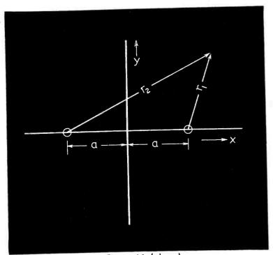
Figure 14 (above) Arrangement of two-wire transmission line. The electrostatic
