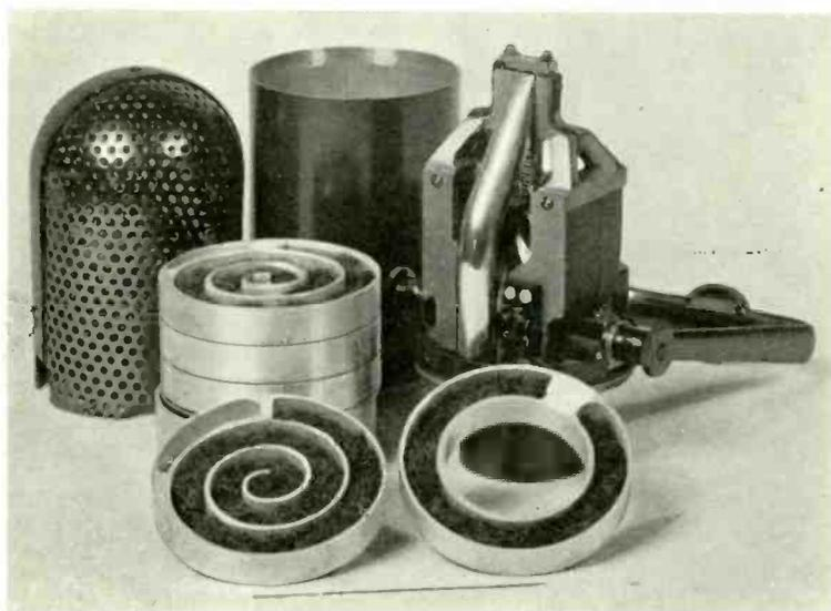
mic pressure in front of the ribbon and the static pressure behind it. In other words, its movement is proportional only to the instantaneous pressure in the sound wave—and it is, therefore, a true pressure microphone.
