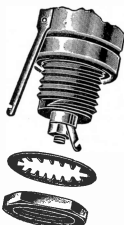
Type G—Grounded Can Mounting Disassembled view of nut, lock washer and screw mounting designed to connect cathode (can) to metal chassis on mounting. Units using this type of mounting can be converted to insulated type mountings by placing an insulating washer over the screw before mounting on chassis.
