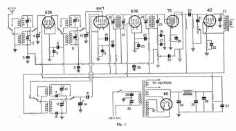
or even less. The reader will also find designs which omit the filter in one or more stages. Generally some kind of filtering will be required where there are two successive stages working at the same frequency.
