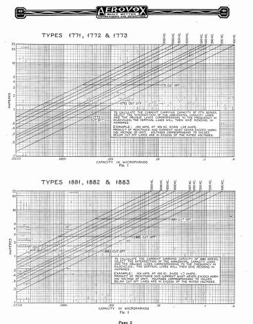
maximum a.c. working voltage for these types are 500 volts, 1250 volts and 2500 volts respectively. The maximum d.c. working voltage of these condensers is 1.4 times as high-700 volts for type 1771, 1750 volts for type 1772 and 3500 volts for type 1773. When the condenser is subject to both a.c. and d.c. voltages, the sum of the d.c. voltage plus the peak a.c. voltage should not exceed the d.c. working voltage rating.
