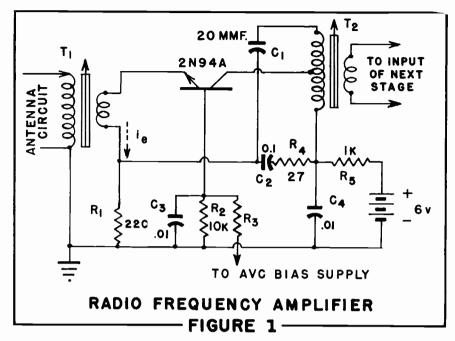
ohms (resistive) and an output impedance of 15,000 ohms. When amplifier stages are cascaded, the interstage transformers (such as  $T_2$ ) must handle this step-down impedance ratio.
