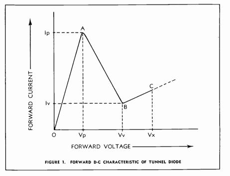
point  $(l_v)$ . And as the voltage is still further increased to  $V_x$ , the current again rises. The conduction curve thus shows two positive-resistance regions (OA and BC) and a negative-resistance region (AB). When the diode is biased into the negative-resistance region, it is capable of oscillation, amplification, bistable switching, or voltage threshold detection in a suitable circuit. Capacitance and capacitor requirements in such circuits are a matter of practical interest.
