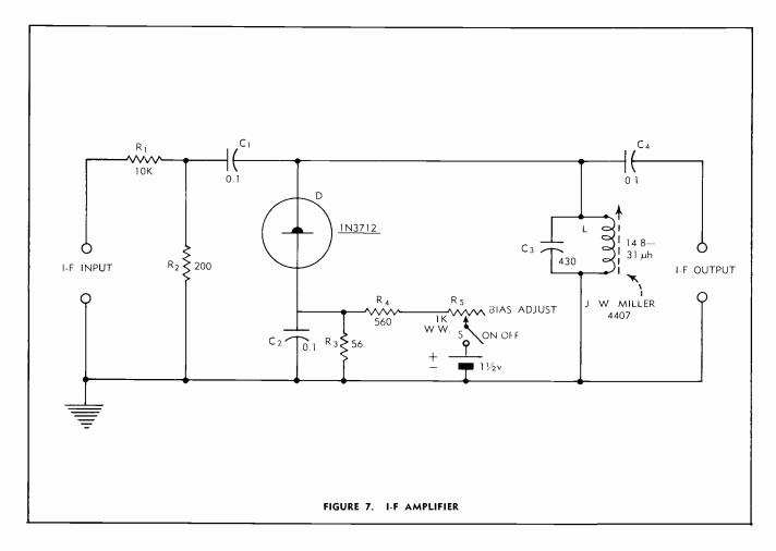
*I-F Amplifier.* Figure 7 shows a 1500-kc intermediate-frequency amplifier which provides a gain of 30 db. It has approximately 200 ohms input and output impedance.
