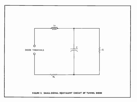
more other frequencies determined by diode internal capacitance, inductance, or negative resistance in combination with stray parameters of some other component. Thus, the internal inductance of a capacitor sometimes sets up a tuned circuit within the capacitor to support "parasitic" operation in a tunnel-diode oscillator. Tunnel-diode a-f amplifiers have been discovered to oscillate at very high frequencies.
