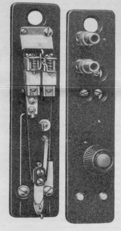
The two strings, which are made of 0.4 mil tungsten wire, as in the case of the single string element, are insulated from each other electrically so that they may be used to observe simultaneously any two different electrical phenomena. An example of this would be to show the phase difference between currents and voltages in different or the same parts of a circuit and so forth. One string may be vibrated at a known frequency to serve as a timing element for the other string.
