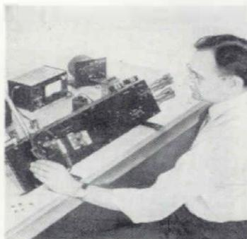
The Transfer-Function Meter described in this issue is a completely new, null-type device, which opens up a new field of measurement. The cover photograph shows the Transfer-Function Meter set up for the measurement of transistors at 400 Mc.
