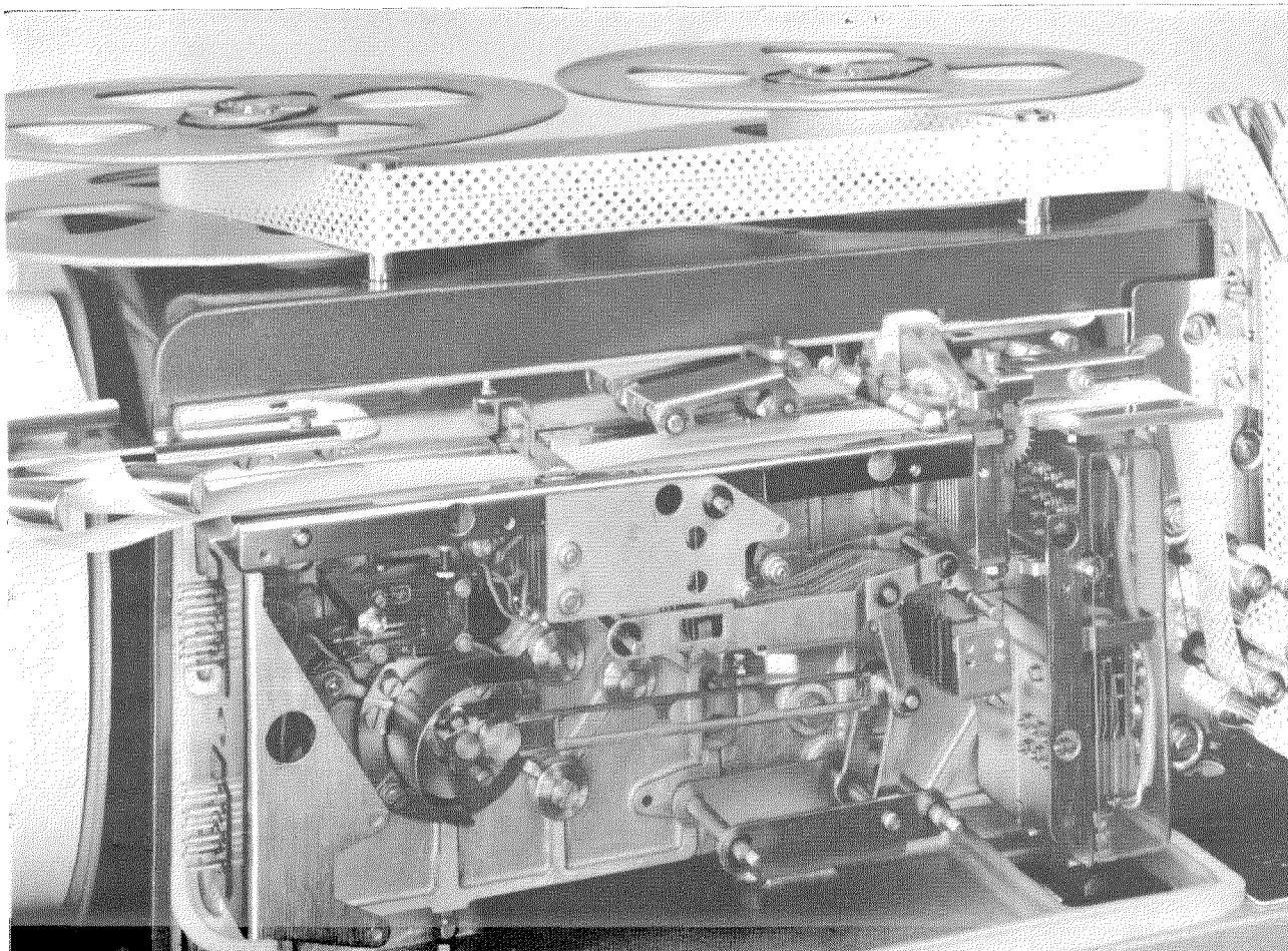
Figure 2—High-speed tape perforator with cover removed.
