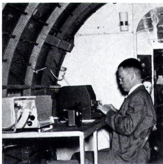
Lightweight Teletype Printer for aircraft shown during demonstration at PICAQ Conference in Indianapolis, 1946, for study of air transportation aids.
