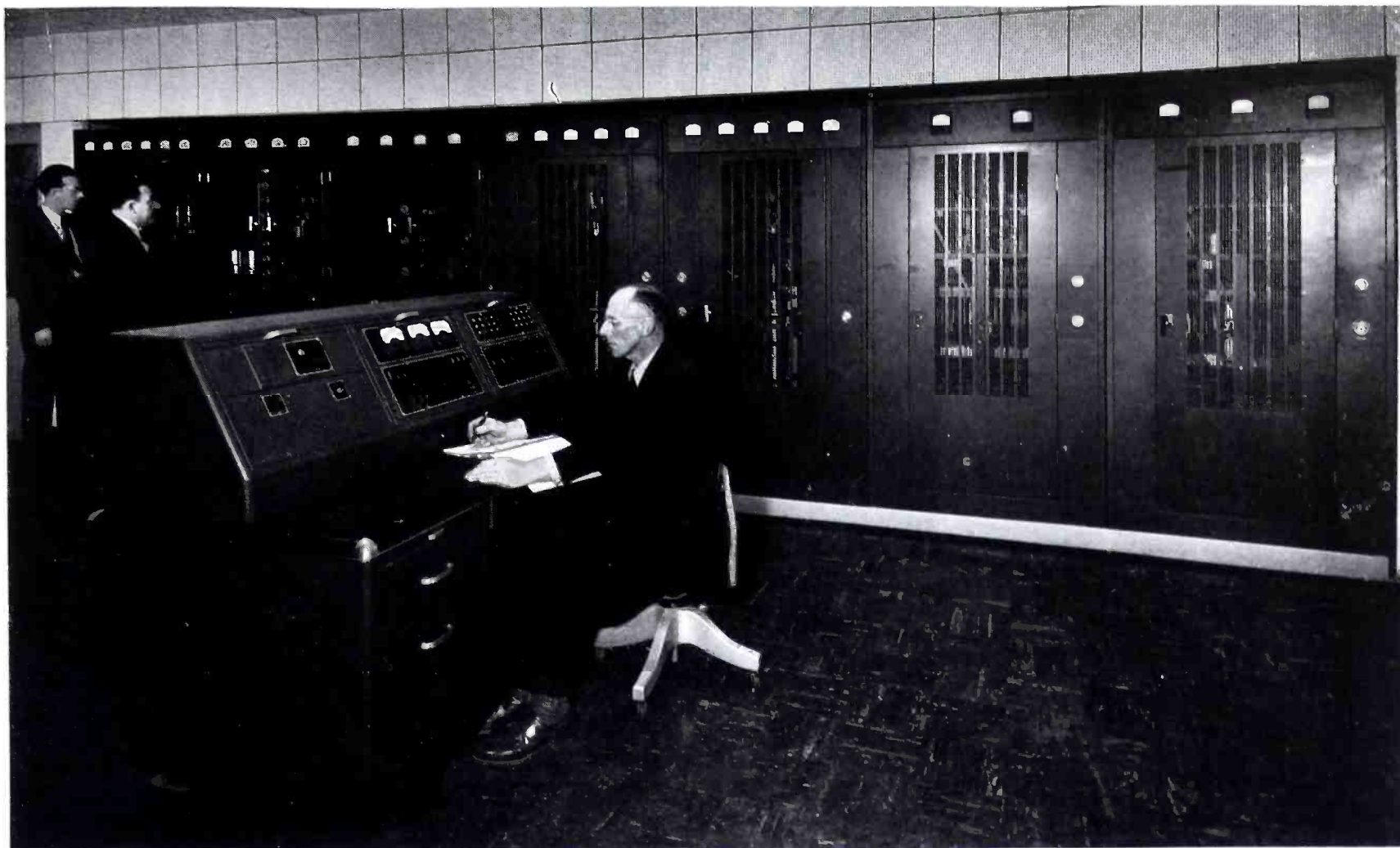
View of KOMA's new 50 kw Western Electric transmitter with KOMA's chief engineer M. W. "Tommy" Thomas seated at the Transmitter Control Desk. This equip-
