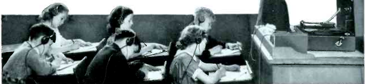
How the Western Electric 4A Audiometer is used to test hearing of New York City children.
