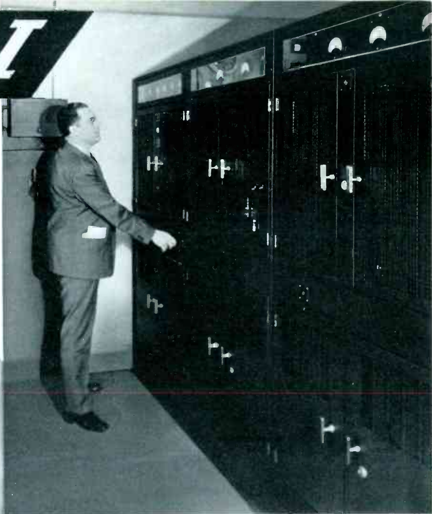
R. J. Rockwell, Technical Supervisor of WLW-WSAI, at the new all AC operated 5 KW Western Electric Transmitter.
