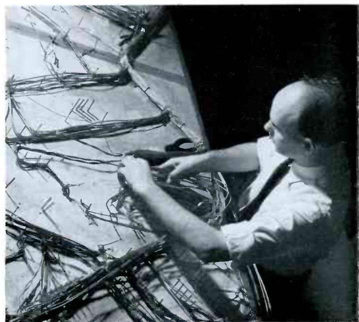
Above: Cable forming like this makes Western Electric transmitters famous for neatness. Below: Assembling 100-250 watt transmitters.
