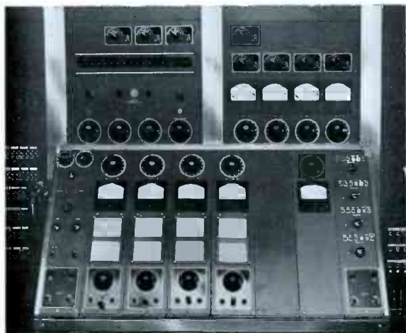
KNX Master Control switching position where the selection and distribution of programs to the CBS networks take place. The new type volume level indicators can be seen here.
