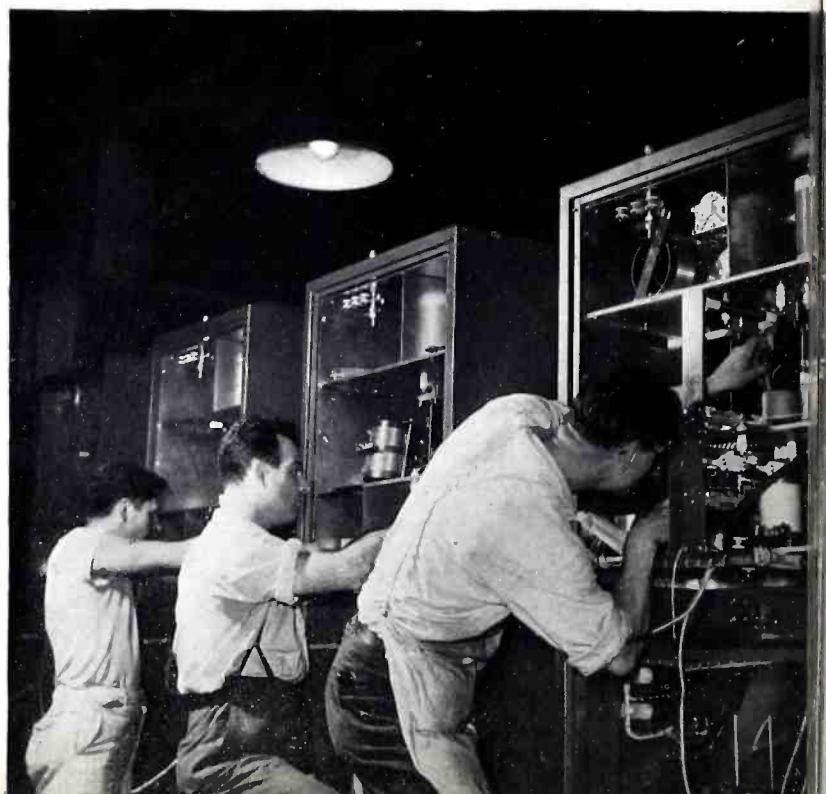
Above: Cable forming like this makes Western Electric transmitters famous for neatness. Below: Assembling 100-250 watt transmitters.
