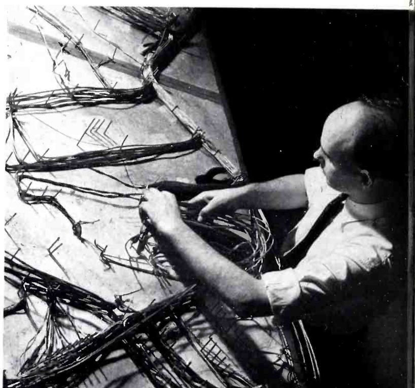
Above: Cable forming like this makes Western Electric transmitters famous for neatness. Below: Assembling 100-250 watt transmitters.
