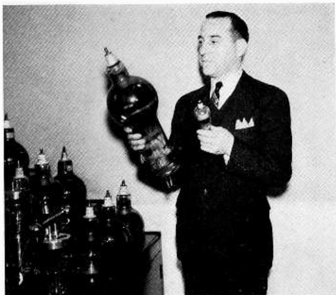
Charles H. Singer displays two of the vacuum tubes which helped make WOR's 1939 record possible. Singer claims that both of these tubes broke all previous records for long life. The larger of the two tubes, a 266B rectifier, burned 33,211 hours before being withdrawn while the 287A had 41,452 hours to its credit. The long life of these, as well as the other tubes in service at WOR, brought this station's 1939 average tube-hour cost down to only $.34.
