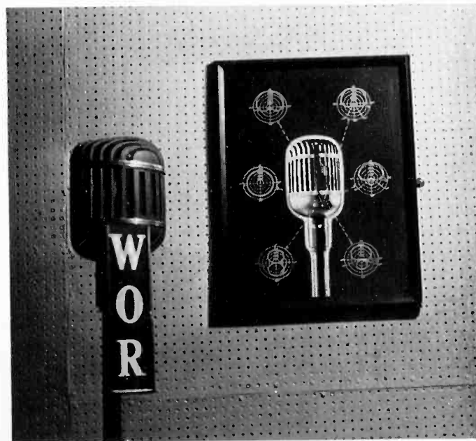
Clipped from the May, 1940, issue of Pick-Ups and mounted on a wall of the control room at the WOR-Mutual Playhouse, this illustration of the six directivity patterns of the 639B cardioid microphone serves a double purpose, according to Playhouse Manager Harry Miller. It serves as a stopper for the enthusiastic production men with definite but mistaken ideas as to how the new microphone should be used. And for those who don't know anything about it but insist on learning, this layout provides a simple explanation.
