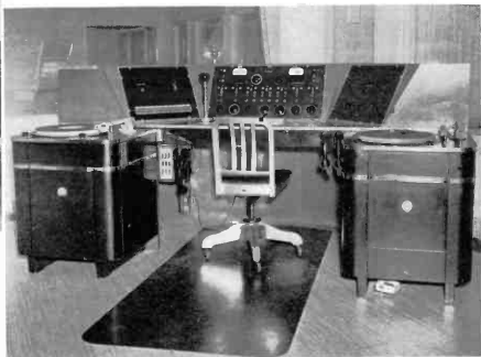
Seated at this control turret the operator has a clear view of both studios and of three racks of speech input equipment.
