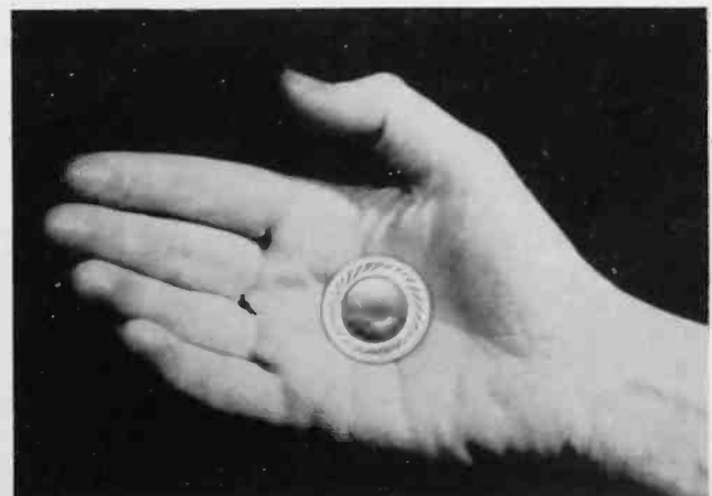
This hand holds the finished diaphragm but no hand touches it at Kearny—vacuum lifts do the handling during forming.
