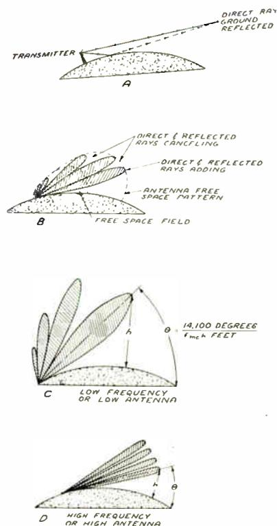
Figure 4—A and B: Radiation striking ground combines with direct rays to increase or cancel strength of free space field, thus dividing energy into lobes. C and D: Number of lobes and height above ground of first lobe depend on transmitter height in wavelengths.
