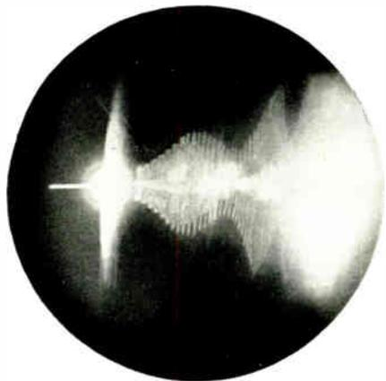
Figure 6—Pattern of voltage built up across opening vacuum switch contacts when 1000 cycle modulation is applied to the 314 kc carrier. Elongated flash across starting spot at left is the return sweep.
