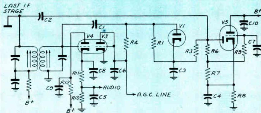
Figure 10—Series delay reducing A. G. C. System.
