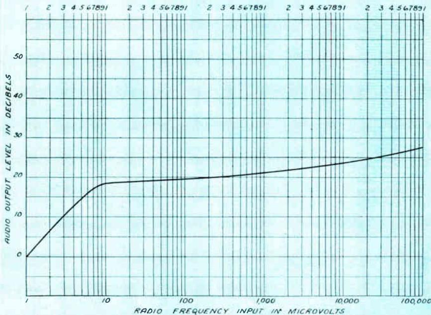
Figure 11—A. G. C. characteristic of series delay reducing system.
