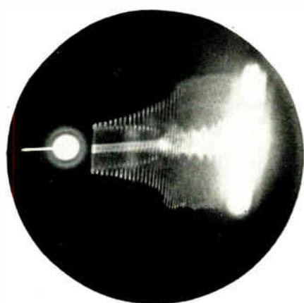
Figure 5—Scope pattern of voltage built up across opening vacuum switch contacts.
