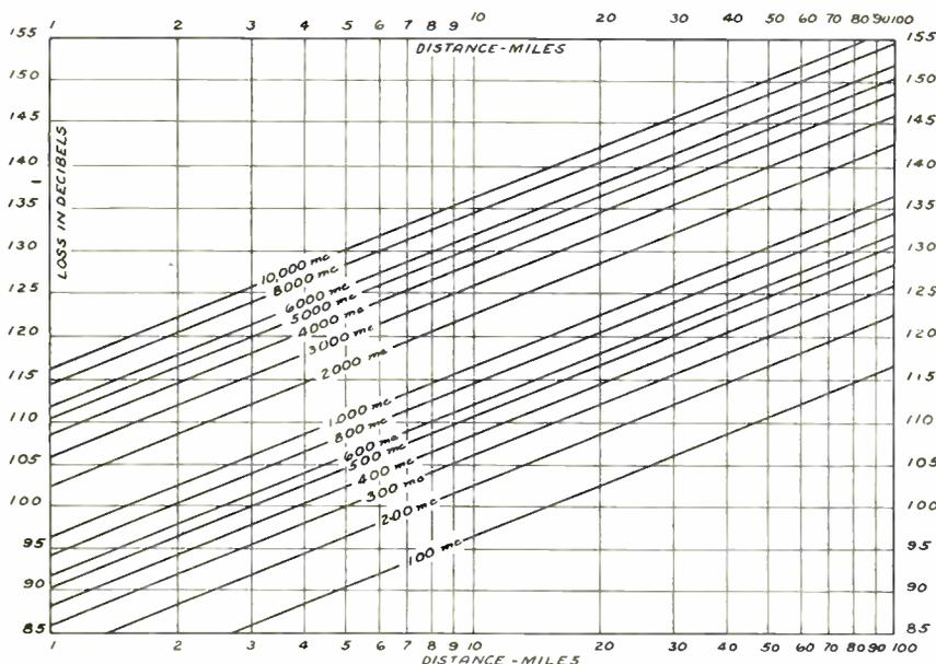
Figure 2—Curves showing circuit losses between two antennas at various distances and frequencies.
