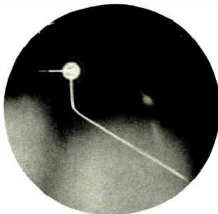
Figure 8—Horizontal sweep starting after the vertical sweep.
