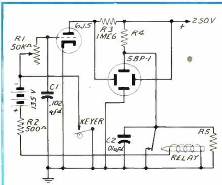
Figure 2—Simplified schematic diagram of sweep circuit No. 1.
