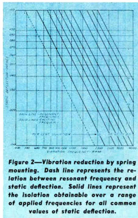
**Figure 2—Vibration reduction by spring mounting. Dash line represents the relation between resonant frequency and static deflection. Solid lines represent the isolation obtainable over a range of applied frequencies for all common values of static deflection.**
