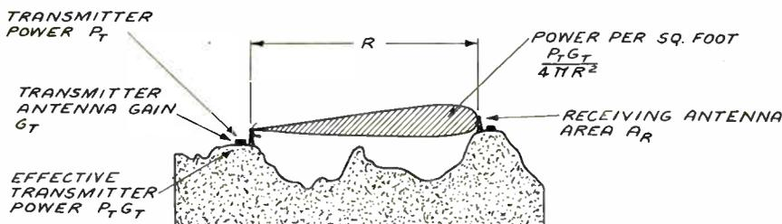
Figure 3—An ideal condition for microwave communication with directional antennas, and an example of power calculations.
