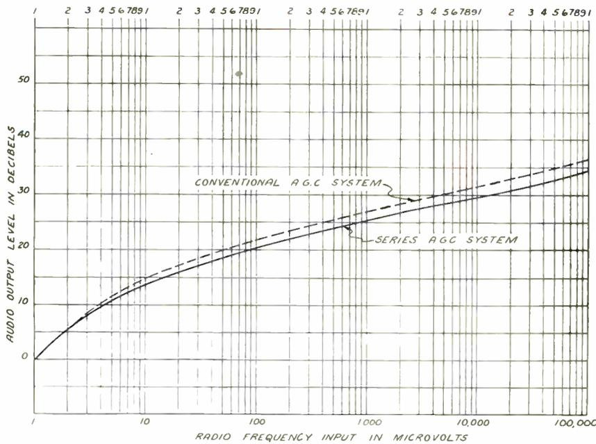
Figure 4—Comparison of A. G. C. characteristics of figures 1 and 2 when bias voltage is applied to amplifier grids.
