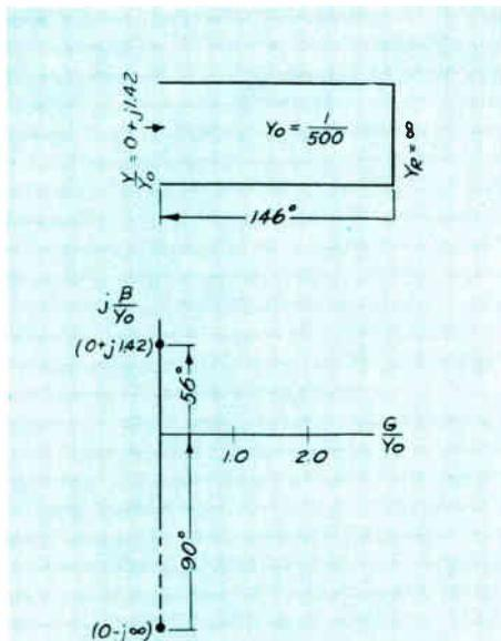
Figure 11—Use of chart to determine stub length.
