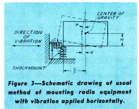
**Figure 3—Schematic drawing of usual method of mounting radio equipment with vibration applied horizontally.**
