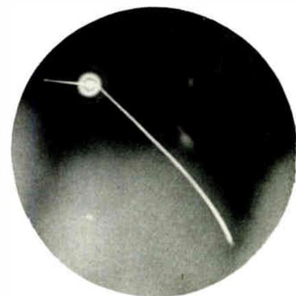
Figure 7—Horizontal sweep starting at the same time the switch contacts open.
