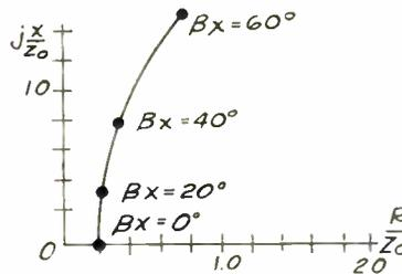
Figure 2—Per unit impedance curve for line terminated in resistance 0.2 times  $Z_0$ .
