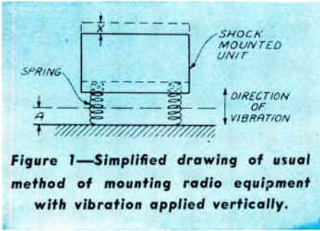
**Figure 1—Simplified drawing of usual method of mounting radio equipment with vibration applied vertically.**
