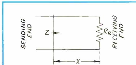
Figure 1—Transmission line terminated in pure resistance.
