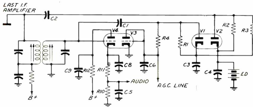
Figure 6—Series delayed A. G. C. system.
