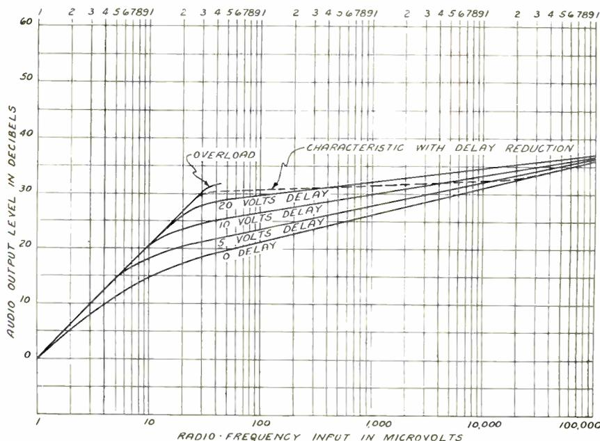
Figure 5—Curves showing improvement in A. G. C. action with delay reduction.
