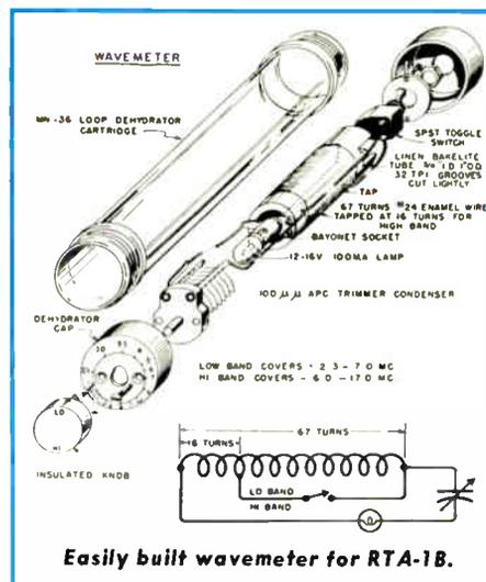
Easily built wavemeter for RTA-1B.
