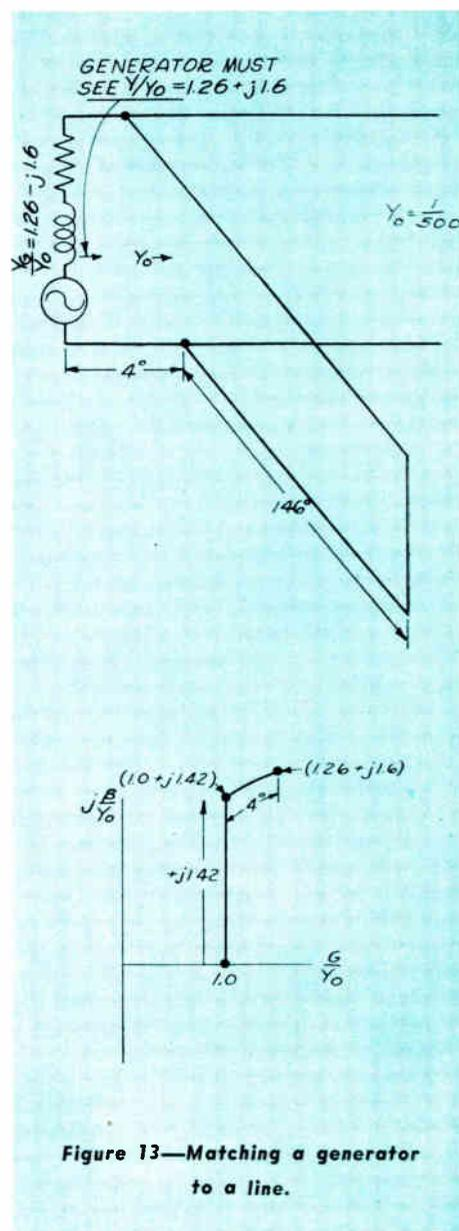
Figure 13—Matching a generator to a line.
