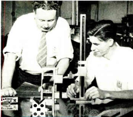
**G. A. Exley, Section Chief, and Bill Britton checking dimensions on a casting with a vernier height gage.**
