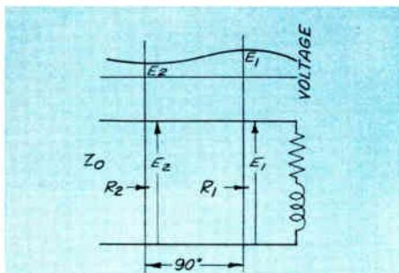
Figure 5—Standing wave of voltage on transmission line.
