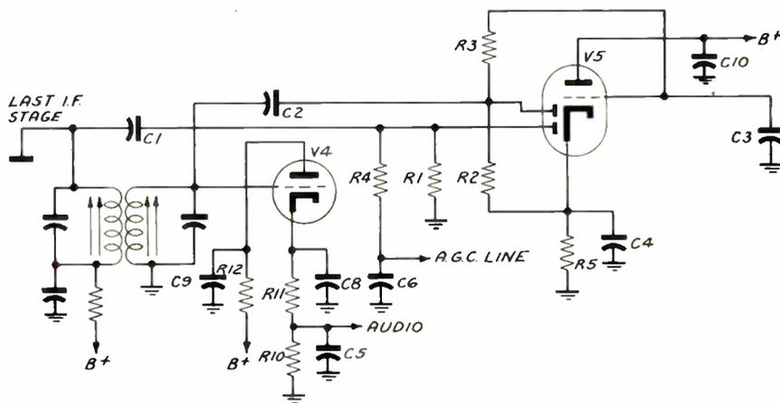
Figure 8—Delay reduction system.
