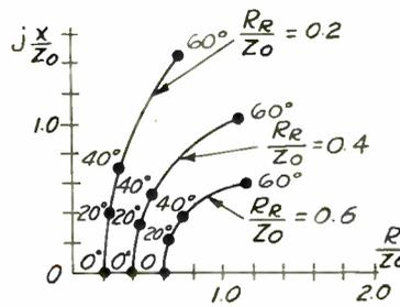
Figure 3—Per unit impedance curves for various terminating resistances.
