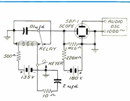
Figure 4—1000 cycle circuit used to time travel of relay armature from unenergized position to closed position.
