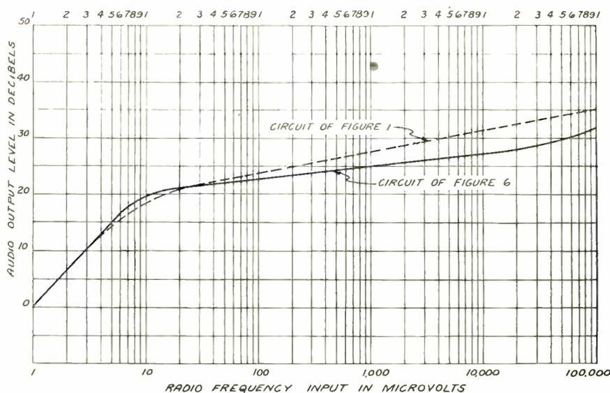
Figure 7—A. G. C. characteristic of circuit in figure 6 compared with that of conventional circuit of figure 1.
