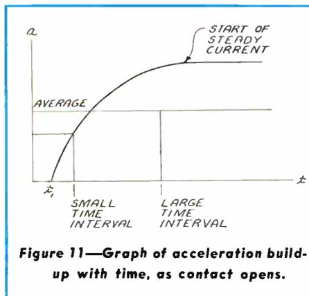
Figure 11—Graph of acceleration build-up with time, as contact opens.
