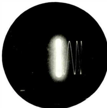
Figure 10—Pattern when 1000 cycle wave is used to time travel of switch armature from the unenergized position to the closed position.
