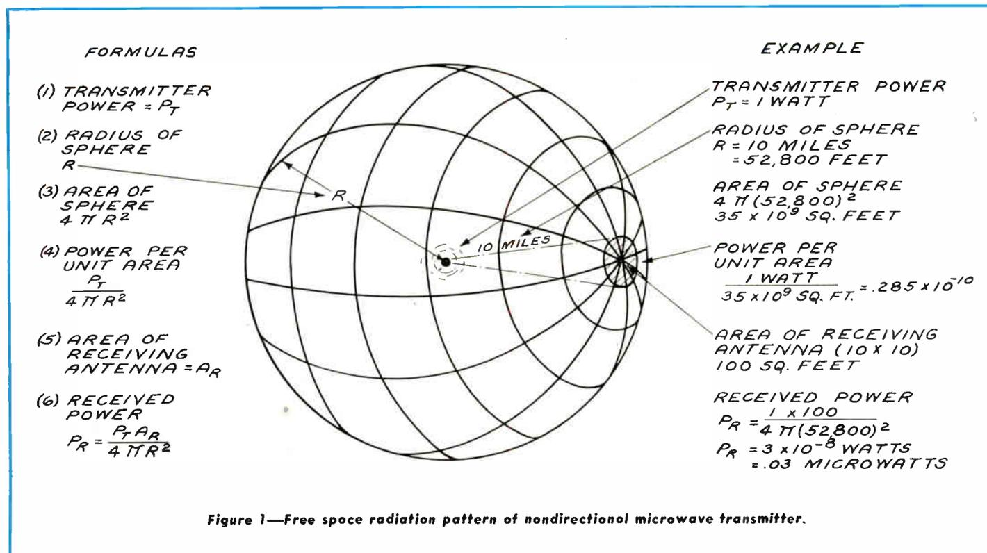
Figure 1—Free space radiation pattern of nondirectional microwave transmitter.
