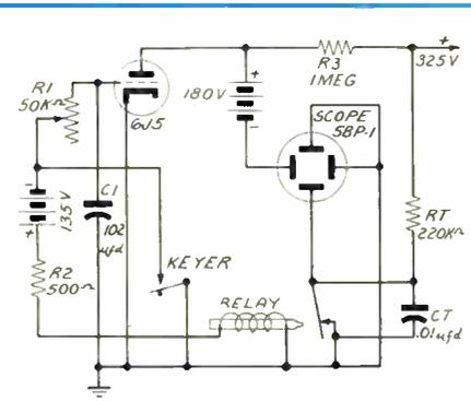
Figure 3—Simplified schematic diagram of sweep circuit No. 2.
