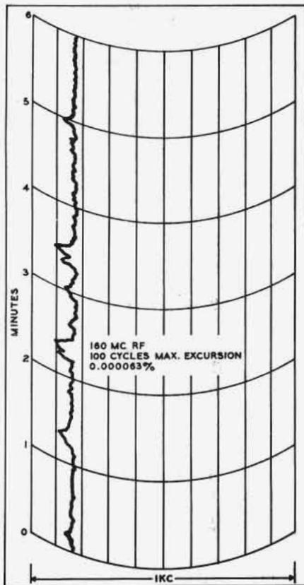
Figure 2. A graphic record of the short-term RF stability of the 225-A.
