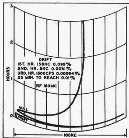
Figure 1. A graphic record of the long-term RF stability of the 225-A.
