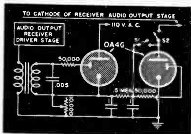
Fig. 4. An alarm system without relays.
