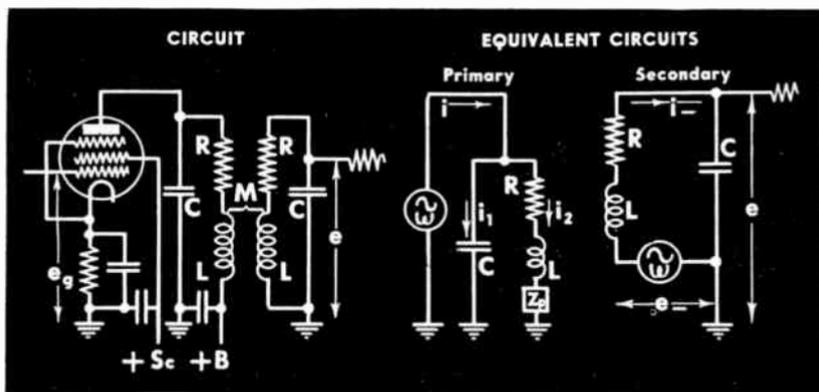
Fig. 1. Universal reference circuit and a simplified equivalent.
