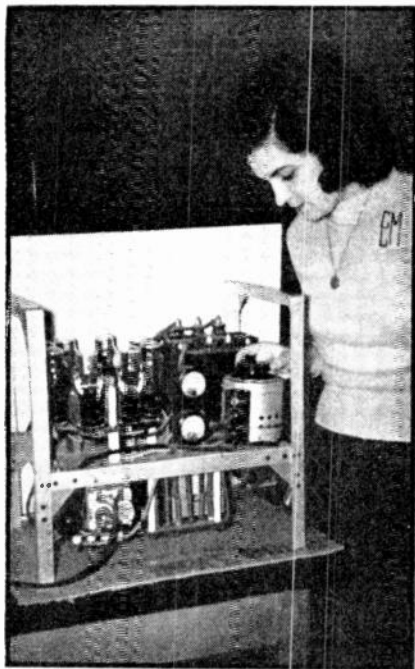
High-voltage bridge rectifier capable of delivering 0.25 amp at 2500 v with eight type 80 tubes. The Variac being adjusted here is connected across the primary of the plate transformer.
