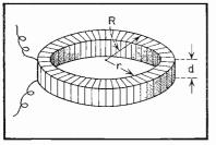
Fig. 4. Dimensions of toroid of rectangular cross section.
