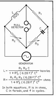
Fig. 6. Circuit of Hay bridge.
