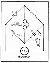
Fig. 5. Circuit of Maxwell bridge.
