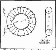
Fig. 3. Dimensions of toroid of round cross section.
