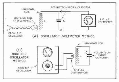
Fig. 7. Resonance methods of checking inductance.
