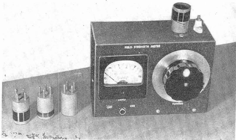
Fig. 1. External View of Transistorized Field Strength Meter. The instrument is self-contained in an aluminum box, 7" long, 5" high, and 3" deep. A single flashlight cell furnishes all power required.
