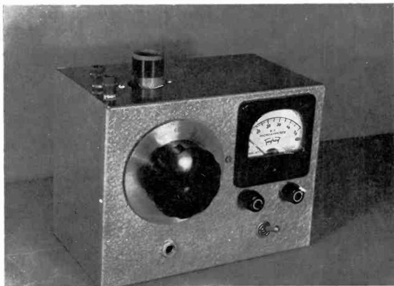
Fig. 1. Completed Modulation Monitor. As shown above, the instrument is built in an 8" x 6" x 4 1/2" aluminum chassis box. It is completely self-contained and transistorized.
