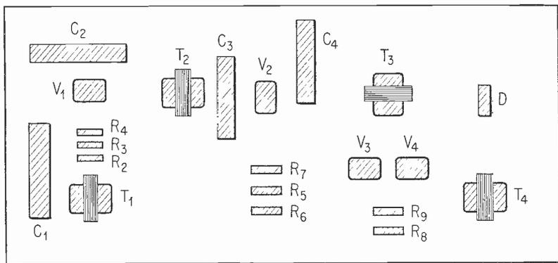
Fig. 4. Circuit Board Layout.
