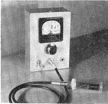
Fig. 1. Transistorized Hum Stethoscope Ready for Use. The hum probe is shown plugged into the input jack, J.<sub>1</sub>. See Figure 8 for identification of components.
