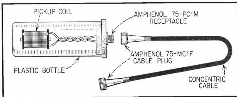
Fig. 7. Details of Hum Probe.
