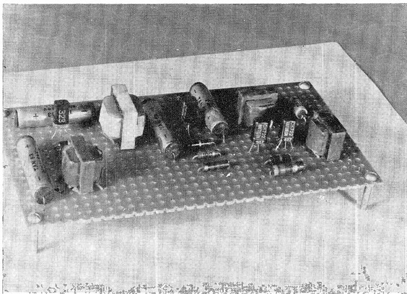
Fig. 3. Completed Circuit Board. Most of the circuit components are mounted on this 6 1/2" x 3 1/2" perforated phenolic board. See Figure 4 for identification of components.
