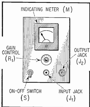
Fig. 8. Front Panel Layout.
