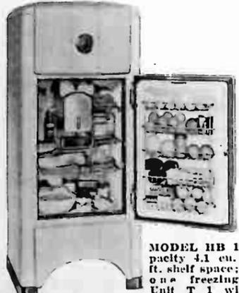
**MODEL HB 1-41**—Net capacity 4.1 cu. ft. 8.33 sq. ft. shelf space; 63 ice cubes one freezing; Hermetic Unit T 1 with still air condenser and other Standard features; Dimensions 53 15/16" high, 23 3/4" wide, 27 3/4" deep. Model HB 3-41 has Standard Q 3 compressor.
