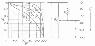
Fig. 3. Effect of alternative method of shunting a linear potentiometer with a fixed resistor
