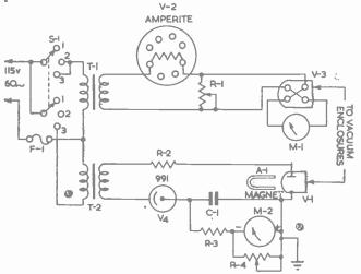
Fig. 21. Combined thermocouple and Penning gauge circuit (Pickard-Smith and Zollard)
