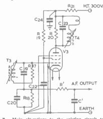
Fig. B. Main alterations to the existing circuit to permit A.M. reception
