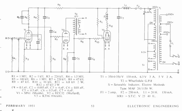
response is restricted somewhat at higher and lower frequencies than 50 c/s., to make instability easier to avoid.
