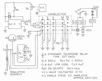
Fig. 1. Circuit details of the analogue computor
