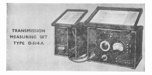
aboratory measurements of the frequency L response of filters, amplifiers, transformers and other components usually require a considerable amount of preparation, involving as they do the use of an oscillator, an attenuator, a valve voltmeter and various change-over switches.
