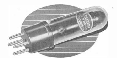
Dimensions: 92 mm seated length, 28 mm diameter and mounted on a four-pin British base.
