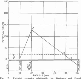
Fig. 17. Potential geometry relationship for Dushman and Found ionization gauge (Reynolds)
