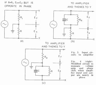
It seems easier to include a resistor  $R_1$  equal to  $R_2$  as shown in Figs. 2 and 3a.  $S_1$  is switched to E and the Y plate also connected to E. This provides a push-pull output with equal and opposite potentials to the X and Y plates for use when setting the pin points, T being disconnected.
