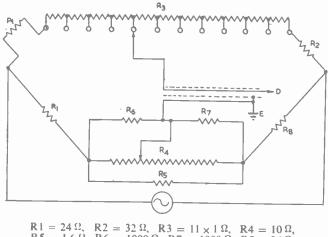
$R5 = 1.6 \Omega$ ,  $R6 = 1000 \Omega$ ,  $R7 = 1000 \Omega$ ,  $R8 = 24 \Omega$ . Pt = 11  $\Omega$  Resistance Thermometer.
