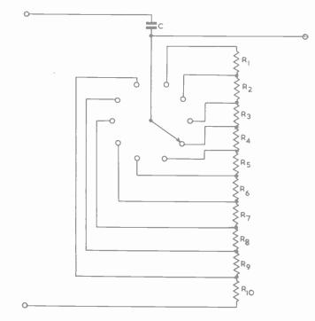
Fig. 6. Circuit Diagram of Variable-Frequency Oscillator  It can be shown that the feedback is given by the expression
