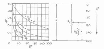
In order to keep the current as small as possible  $R_2$  and hence  $R_1$  should be as large as possible.
