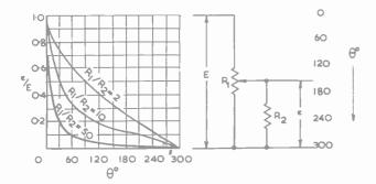
Fig. 1 shows the characteristic obtained by normal use of a linear potentiometer, and for comparison, the curve of a logarithmic potentiometer of well-known manufacture.
