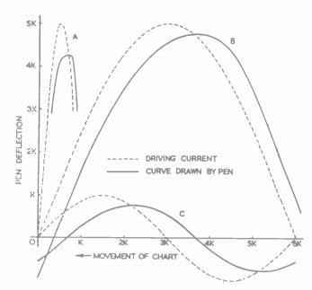
Fig. 5. The effect of static friction on the response of a pen recorder (computed)
