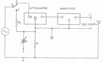
Fig. 2. Modified circuit to measure voltage gain and phase shift
