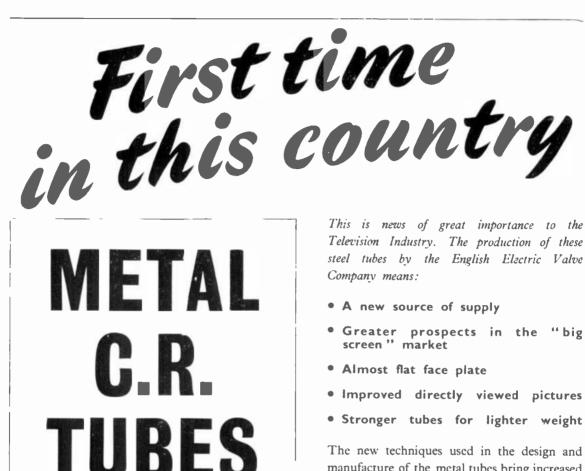
The new techniques used in the design and manufacture of the metal tubes bring increased picture brightness, improved picture detail resolution, good contrast even under high ambient light conditions, and a large screen area in relation to face area. Size of tube 16" diameter.
