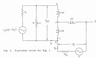
the leakage inductance may have a first-order effect on the phase-shift. Any self-capacitance or other stray capacitance may be included in the term X in Equation (2). It is clear that the anode-to-cathode coupling, which produces negative voltage-feedback, gives the effect of a low internal resistance in the valve, since the greater the amplification factor ( $\mu$ ) the smaller the phase-shift becomes.
