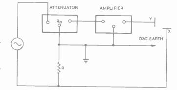
Fig. 1. Usual circuit to measure voltage gain
