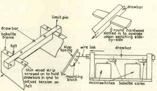
Fig. 22. Stop switches using microswitches
