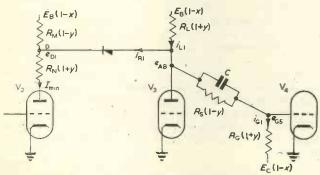
Fig. 9. Limits for determining RM and RN
