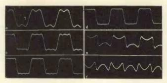
Fig. 8. (a) Synthesis of square wave: Fundamental+3rd harmonic; (b) Fundamental+3rd and 5th harmonics; (c) Fundamental+3rd, 5th and 7th harmonics; (d) Fundamental+3rd, 5th, 7th and 9th harmonics: (e) As (d) but with fundamental amplitude reduced; (f) As (d) but with fundamental suppressed.
