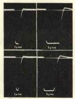
Fig. 3. Gating pulses of 1 and  $3\mu$  sec duration
