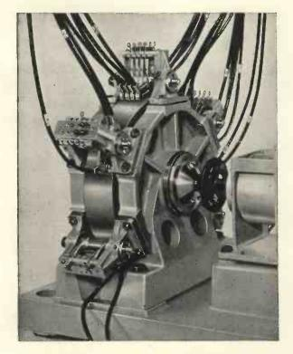
For the drum, which is the main store or memory of the computer, a metal was required with sufficient homogeneity for symmetrical turning to obviate the need for balancing and which would thereafter remain stable. 'Duralumin' was the answer.
