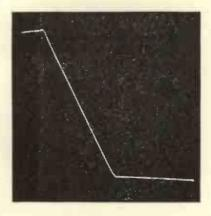
Fig. 9. 1·25μsec. 450V sweep, from push-pull generator, 1 000 sweeps superimposed
