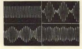
in Fig. 11(b), in which the upper sideband is represented as a vector rotating at fundamental frequency in an anticlockwise direction. The resultant of the two sidebands consists of a stationary vector parallel to the carrier, the length of which varies sinusoidally at fundamental frequency. The depth of modulation is seen to be 80 per cent.
