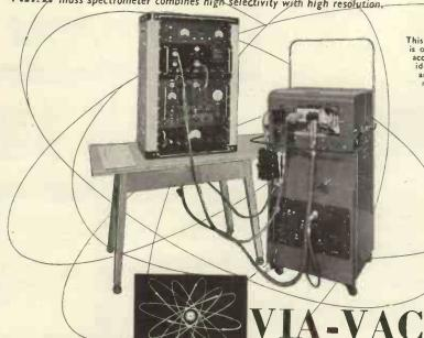
This mass Spectrometer is of high sensitivity and accuracy, and provides identification of inorganic and organic molecules of mass numbers 16—90. The minimum of variable controls thoughout the full scale of recording, contributes towards trouble-free service. The Spectrometer is of the 180° focussing type with fixed magnetic field of 1500 Gauss and a varying accelerating voltage.
