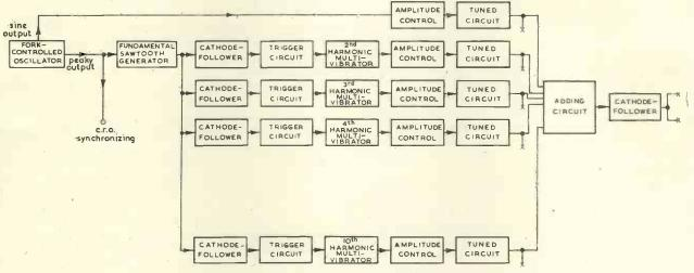
Fig. 1. Arrangement of the synthesizer
