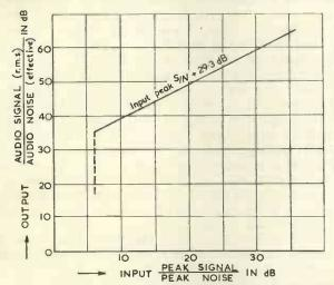
Fig. 2. Theoretical signal-to-noise ratio in p.l.m.
