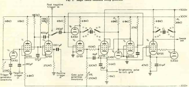
Fig. 2. Single ended feedback sweep generator
