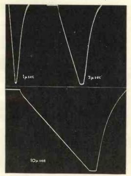
Fig. 4. Sweep waveforms from single ended sweep generator of 1, 3, and  $10\mu{\rm sec}$  duration
