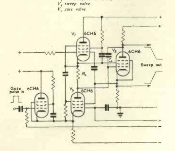
improvement would be to use a valve type such as the CV2127 (6CH6) throughout as the pentodes drawn, as these valves have much smaller inter-electrode capacitances than the CV173 (EF55) and will pass considerably more current than the CV138 (EF91) within their negative grid base.
