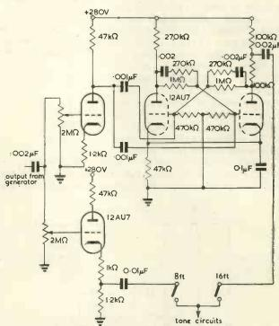
Fig. 25. Frequency divider and isolating valves
