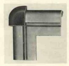
As will be seen from the illustration the triple-pronged corner-connector corresponds in section with that of the frame-Thus these two units interlock precisely and simply. Allowance is, of course, made for screw tapping or similar fixing: and the rebated edge on the frame-member provides for a clean flush fitting of panels of any suitable material.
