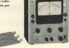
The accuracy is better than 0.03% for indication round the zero point and better than 3% for full scale indication of impedance or phase angle deviations.
