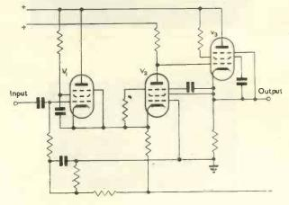
impedance for the input signal, while V2 provides a cathode-follower output capable of driving the screen and suppressor grids of V<sub>2</sub> to follow the rise of its anode voltage, in order to allow the latter to rise at the maximum possible rate once the valve has been cut off by the rising edge of the input waveform.
