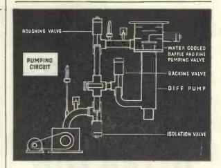
Fully automatic and protected pumping plant for sequence pumping
