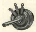
STANDARD CARBON POTENTIOMETERS. Made by an entirely new method ensuring a highly stable resistance element, which is also very durable. Silent and smooth in operation, these controls offer both mechanical and electrical reliability. Soldering tags are heavily silver plated to resist oxidisation, and the mains switch has an efficient quick make-and-break action.
