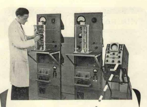
In common with most large manufacturing concerns, the MARCONI-OSRAM VALVE CO. employs Cossor Oscillographs to help investigate vital manufacturing problems. The picture shows a "Q Series" Valve Vibration Rig where stresses of known form, amplitude and frequency are applied to valve samples to simulate accurately their mechanical conditions of service.
