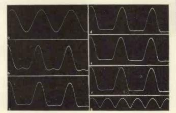
Fig. 7. (a) Fundamental; (b) Fundamental+2nd; (c) Fundamental+2nd+4th; (d) Fundamental+2nd+4th+6th; (e) Fundamental+2nd+4th+6th+8th; (f) Fundamental+2nd+4th+6th+8th+10th; (g) Half-wave rectified sine-wave with fundamental suppressed
