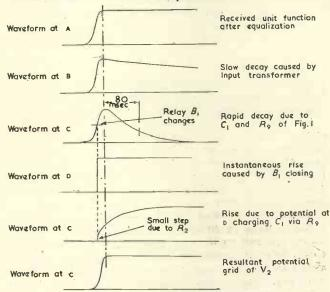
Fig. 2. Waveforms in circuit when unit function is received
