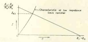
Fig. 12. Construction for determining In-
