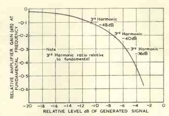
Fig. 6. Measured relationship between amplifier gain at the fundamental frequency and the amplitude of the generated signal
