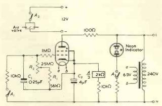
Fig. 6. Circuit used to provide automatic artificial respiration
