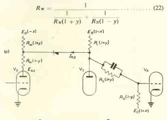
Fig. 11(a). Limits for checking lowest grid potential of a conducting valve
