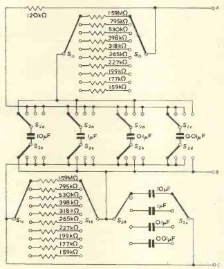
Fig. 5. Circuit of frequency control network ±1 per cent tolerance on component values.
