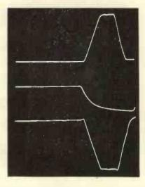
Fig. 10. 1-25 µsec push-pull generator waveforms displayed on a 10 µsec horizontal timebase
