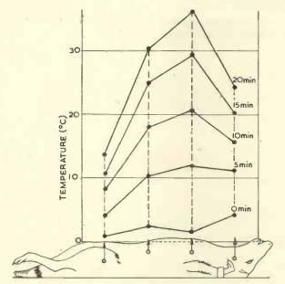
Fig. 4. Temperature rise plotted for different sections of a rat corpse when placed in the beam
