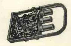
'Duralumin' is used in the construction of the 223 plug-in units which form the main feature of the 402 computer.
