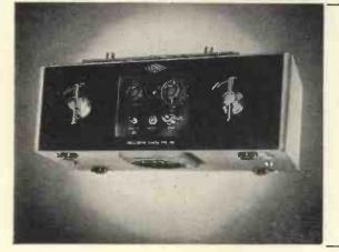
THE OSCILLOSCOPE CAMERA TYPE 758 is designed specifically for use with Airmec Oscilloscopes. It may be used for single shot photography or continuous recording, and a motor with variable speed gearing is included for the latter purpose. The cassettes will accommodate 100 feet of 35 mm. film or paper and a footage indicator shows the amount of
