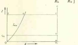
Fig. 10. Construction for determining RM and RN
