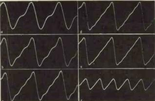
Fig. 9. (a) Fundamental +2nd; (b) Fundamental +2nd+3rd; (c) Fundamental +2nd+3rd+4th; (d) Fundamental +2nd+3rd+4.h+5th; (e) Fundamental +2nd+3rd+4.h+5th; (f) Fundamental +2nd+3rd+4.h+5th; (e) Fundamental +2nd+3rd+4.h+5th; (f) Fundamental +2nd+3rd+4.h+5th; (e) Fundamental +2nd+3rd+4.h+5th; (f) Fundamental +2nd+3rd+3rd+4.h+5th; (f) Fundamental +2nd+3rd+3rd+4.h+5th; (
