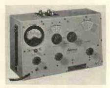
directly in terms of circuit magnification. The oscillator is modulated at 50c/s 50 per cent, so that d.c. amplifiers need not be used in the valve voltmeter, thus eliminating zero setting.
