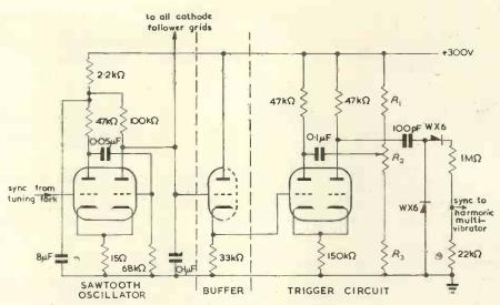
Fig. 3. Phase controlling unit
