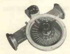
incorporates a unique means of compensation of the scale reading to correct the variation with frequency in attenuation characteristic of the metallised vane within the guide. There is no need to refer to calibration data and errors due to incorrect setting up are virtually impossible.
