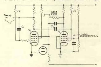
Fig. 1. Suppressor gated sanatron sweep generator  $V_1$  sweep valve  $V_2$  gate amplifier
