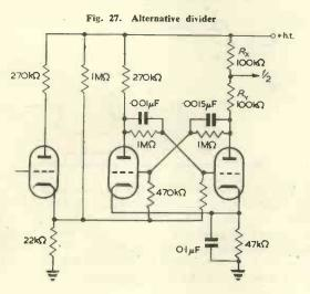
values of  $R_x$  and  $R_y$  can be adjusted to set the level. The divided signals can be injected into the grid of the 6BA6 valve and another way of doing this is to tap the unison, 8ft and 16ft signals into a potential divider between the grid of this valve and earth, at points found by trial. These points are switched to isolate any particular pitch not required.
