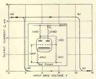
Fig. 3. Measured transfer characteristic of Schmitt-Trigger circuit
