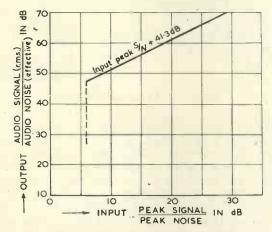
Fig. 3. Theoretical signal-to-noise ratio in p.p.m.
