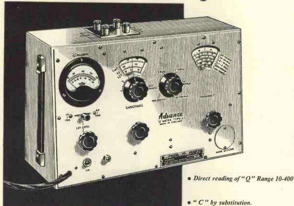
The ADVANCE "Q" Meter is different! It is small, portable and has an excellent specification—a useful addition to any electronic laboratory and well suited for production testing. Furthermore, it is offered at a price to suit all applications. With the T1, RF measurements can be made of "Q" inductance, impedance, capacitance and power factor at frequencies between 100 kc/s. and 100 Mc/s.
