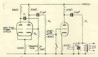
Fig. 4. Harmonic multivibrator and output stage
