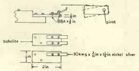
Fig. 14. Octave coupler key wipers and contact wires.
