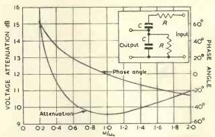
Fig. 1. Attenuation and phase angle/frequency characteristic of basic frequency control network at a given setting  $\omega_{\rm o}=1/CR$
