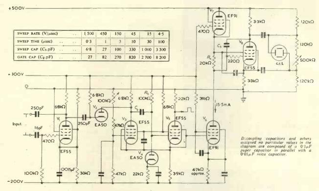
Fig. 6. Push-pull feedback sweep generator
