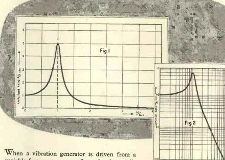
When a vibration generator is driven from a variable frequency source of supply, the amplitude response will be as shown in Fig. 1, for a
