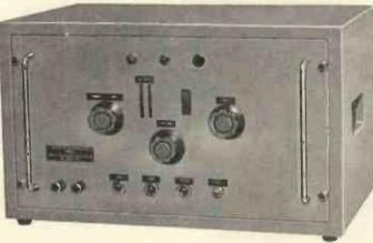
MOTOR OR MANUAL DRIVE AT WILL. FREQUENCY RANGE 20cs. TO 3Kcs.
