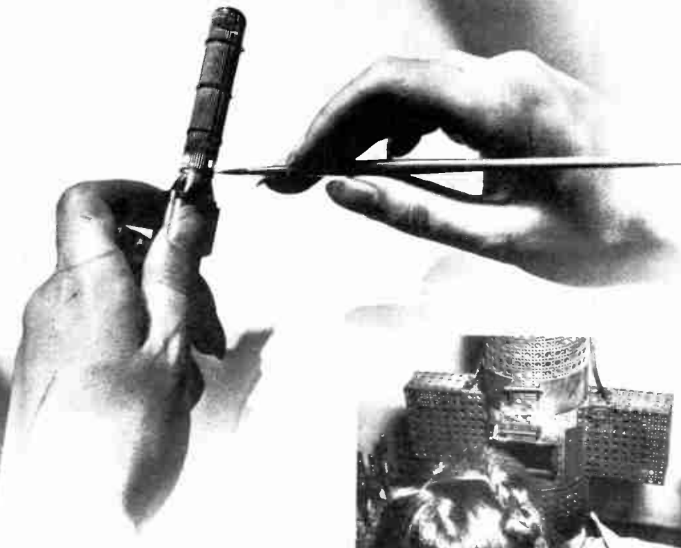
Alloy flows easily and weld is quickly completed under arc.
